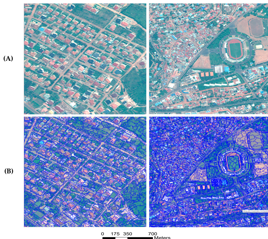
Figure 3. Excerpts of segments generated from WV-2 image. Row (A): the original WV-2 with natural color display (red, green and blue bands' combination); Row (B) represent the generated segments in the two corresponding areas.
