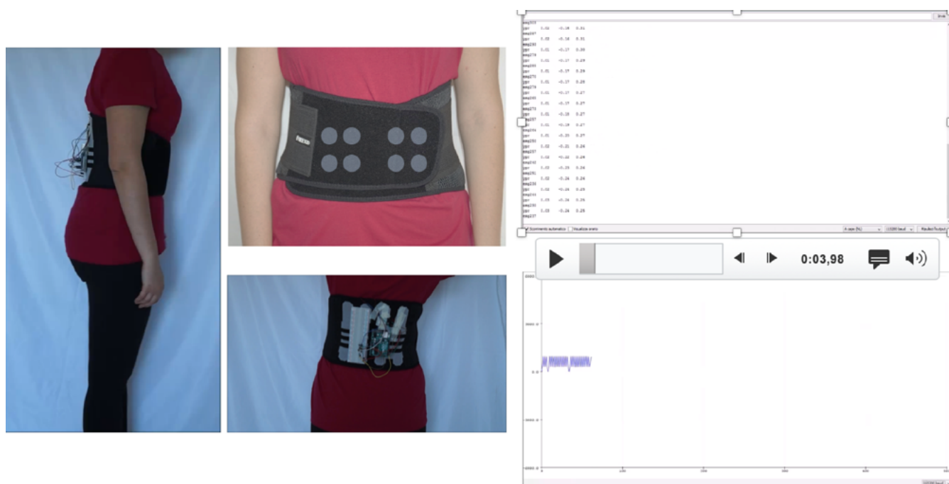
Fig. 6. This image captures the functioning of the prototype. On the right you can see the IMU sensor data movement and the muscle extension monitoring by EMG sensors.
