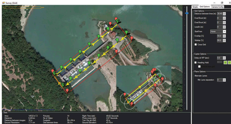
Figure 5. Flight planning realized by Mission Planner software for a quadcopter UAS mission.
