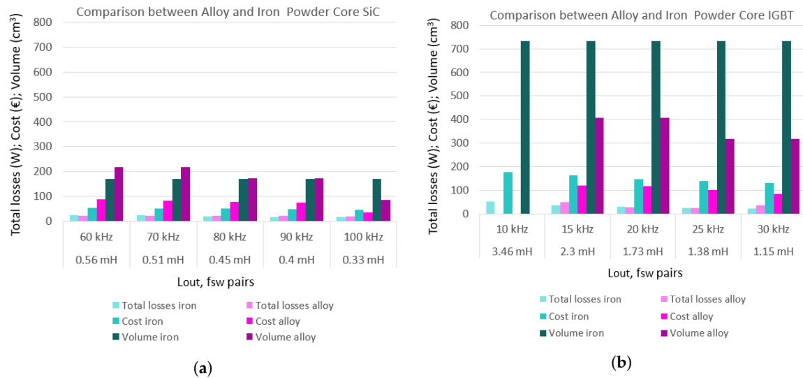
Figure 5. Comparison of cost, volume and total calculated losses for iron and alloy powder cores: (a) SiC-MOSFET-based converter; (b) Si-IGBT-based converter.
