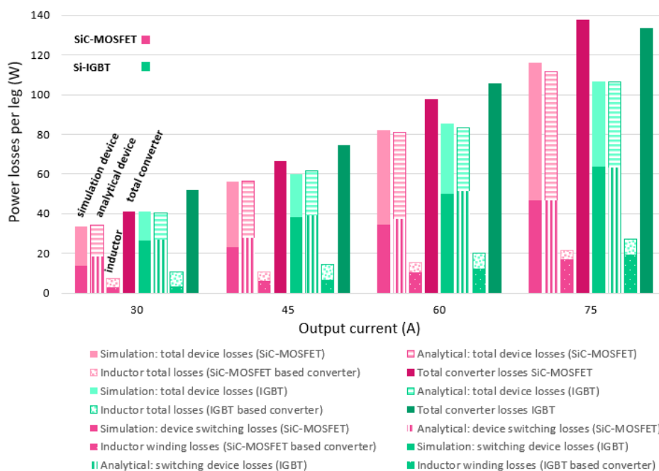
Figure 9. Loss distribution for 0.45 mH–80 kHz and 1.73 mH–20 kHz pairs and comparison with analytical values.
