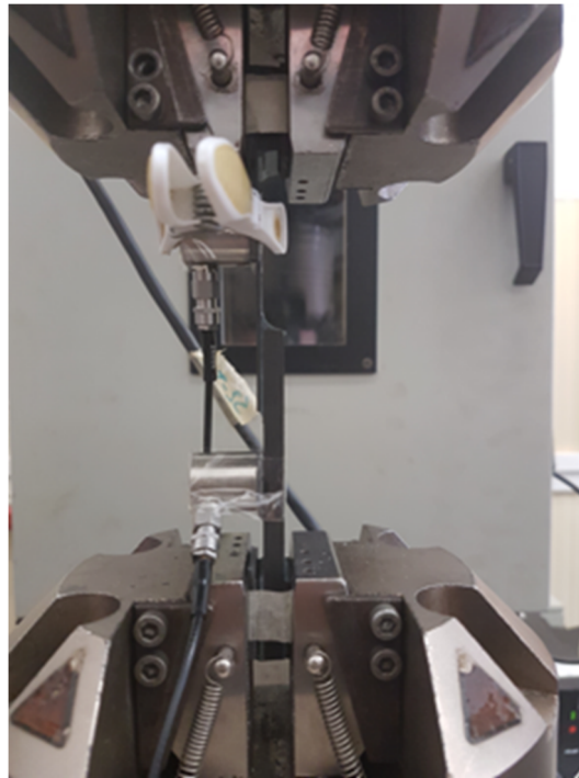
Figure 2. Testing setup with SLS specimen mounted along with the Acoustic Emission (AE) sensors.
