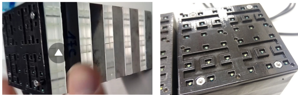
Fig. 6. PLAS reference calorimeter. Left: the absorber-scintillator stack before wrapping with black tape. Right: a detail on the 3D-printed mask used to interface the WLS fibers and the SiPM mounted on the PCB.
