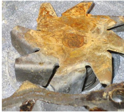
Figure 1.2. Rust and Corrosion [2].
