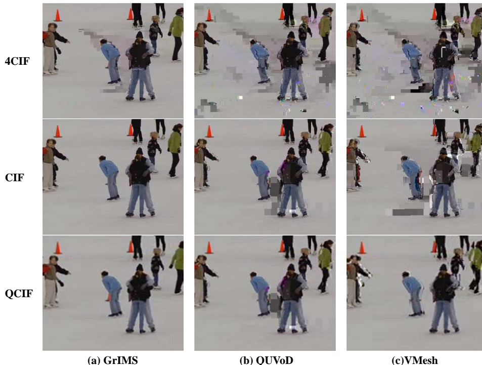
Fig. 15. Frames taken from received and reconstructed videos with three different formats by (a) GrIMS (b) QUVoD (c) VMesh
