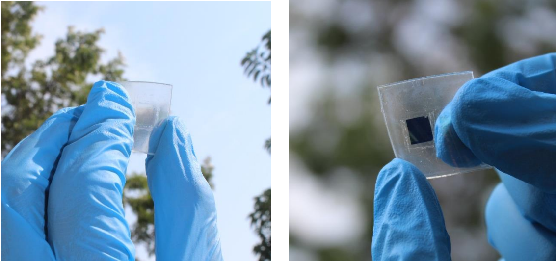
Fig. 3. Pictures in bleached and colored conditions of flexible EC devices fabricated on polyethylenenaphthalate (PET) substrate.
