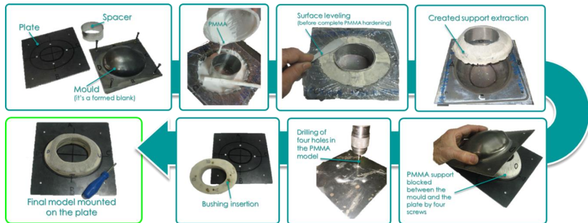
Figure 7. Procedure of support manufacturing.
