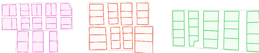
Figure 6.6.3 - Example of the most recurrent masonry building aggregate configurations of the C02 urban sector
