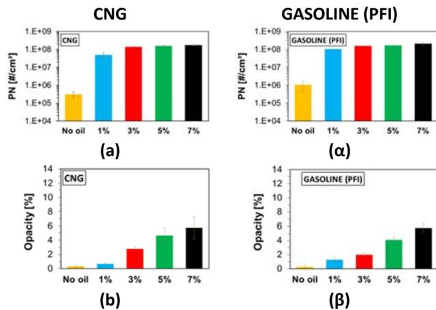
1 **Figure 8** Total concentration number for CNG (a) and gasoline ( $\alpha$ ); opacity [%] for CNG (b) and gasoline ( $\beta$ ) tests.
