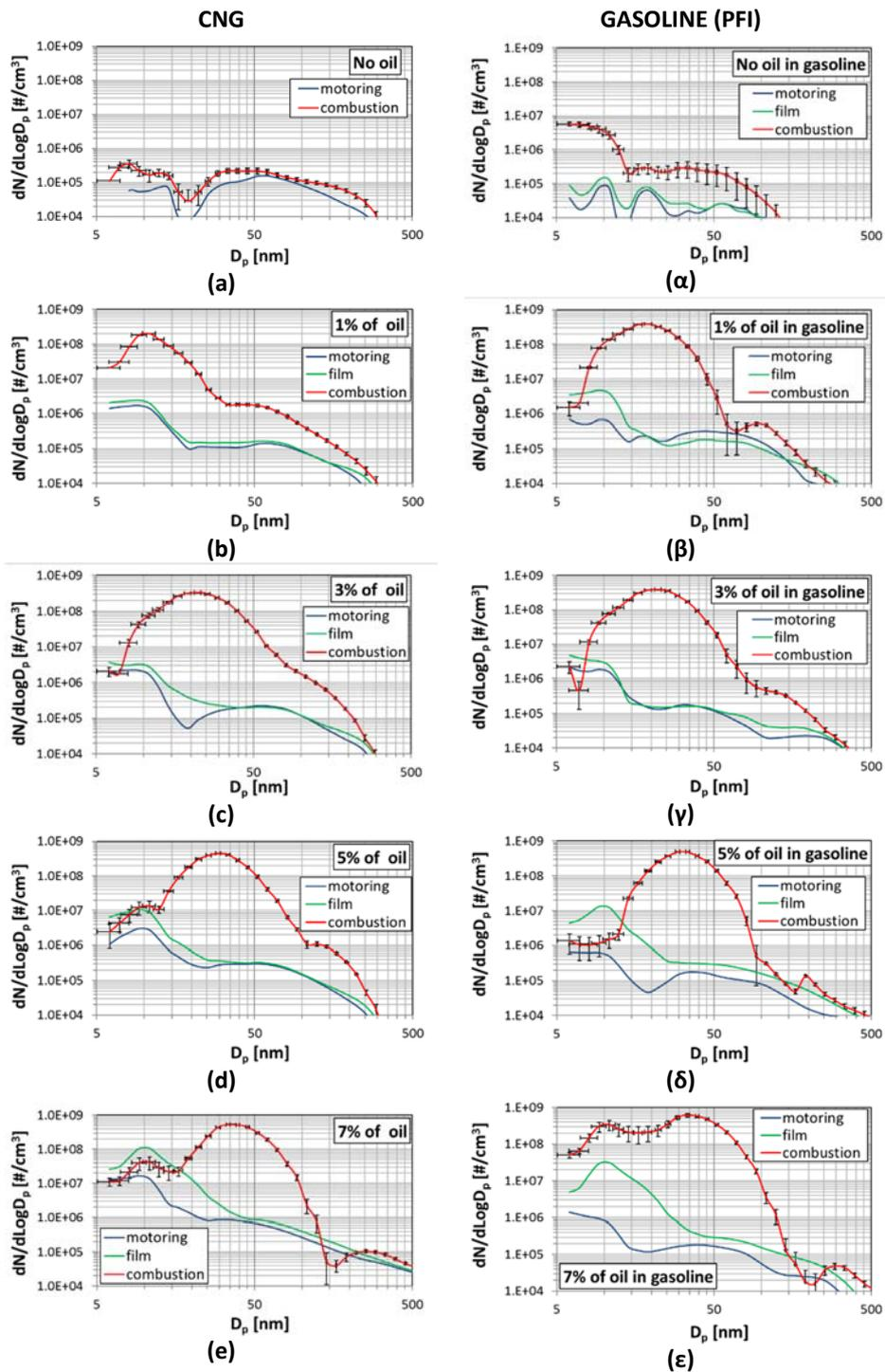
12 **Figure 6** PSD functions for one representative case for each explored operating condition for both the CNG (Latin
