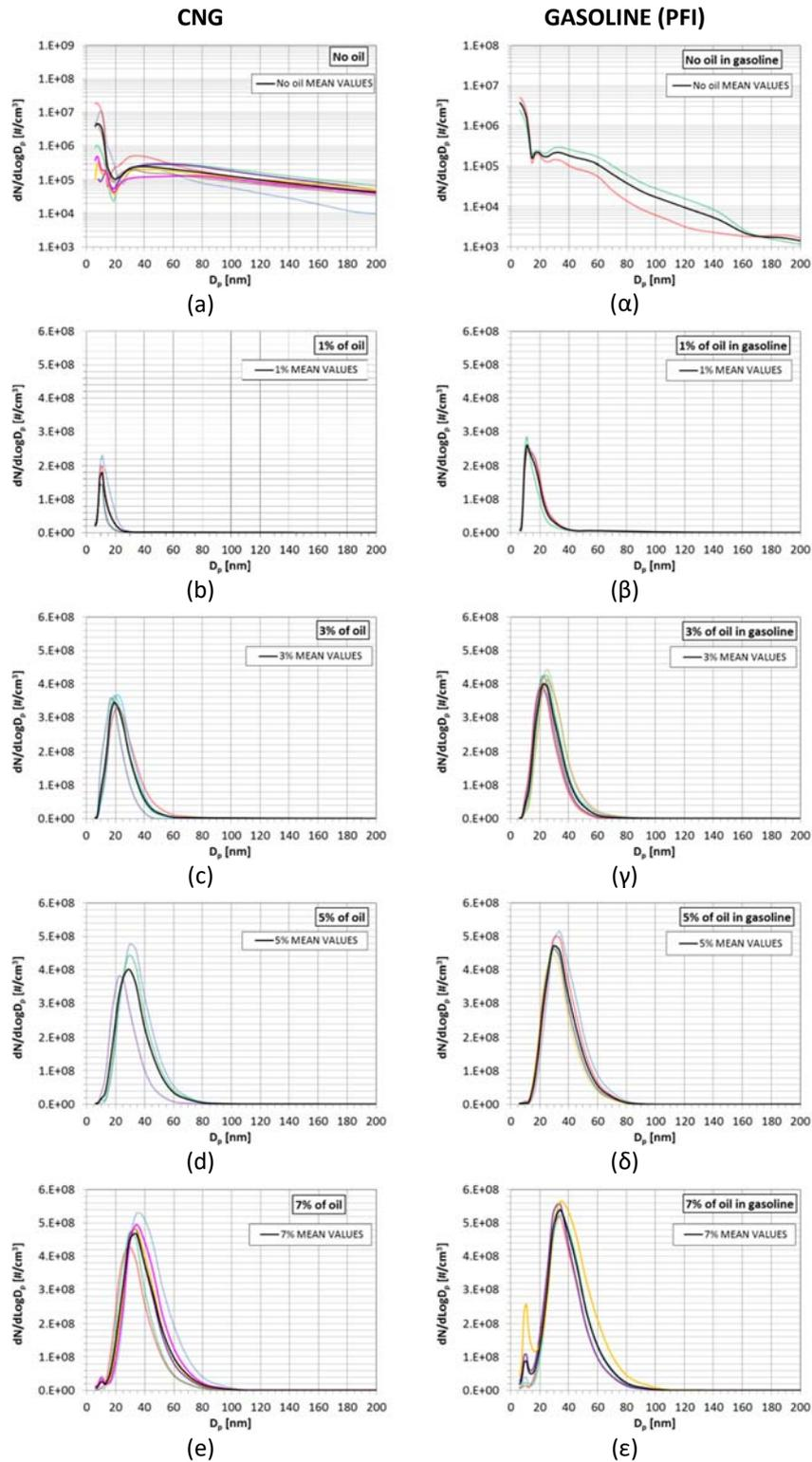
1 **Figure 4** Statistical data concerning the PSD functions measured for both CNG (Latin characters) and gasoline (Greek characters) PFI tests. In each graph, the distributions obtained from each repetition of the same test are reported,
