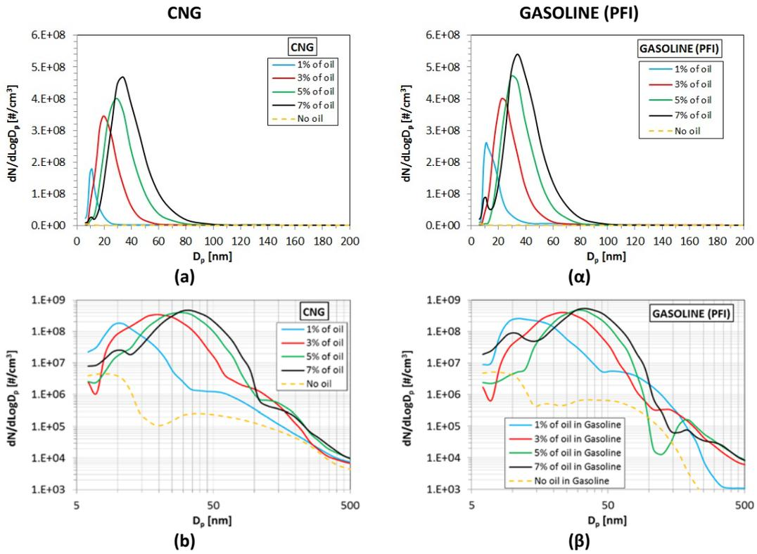
6 **Figure 7** PSD functions (mean values) with a mass lubricant oil content equal to 0% (yellow line), 1% (light blue line),
