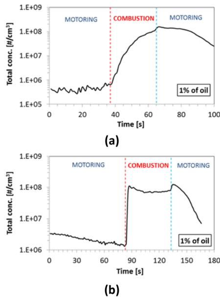
26 **Figure 3** Total PN concentration measurements for CNG test with 1% of oil without (a) and with (b) “film-strategy”.
