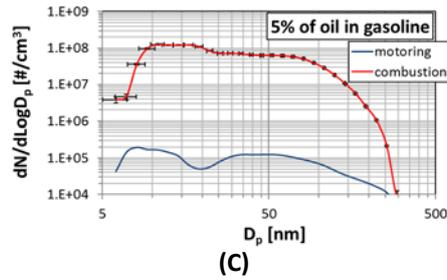
1 **Figure 9** Statistical PSD functions (a), total concentration number trace evolution with time (b) and PSD functions
