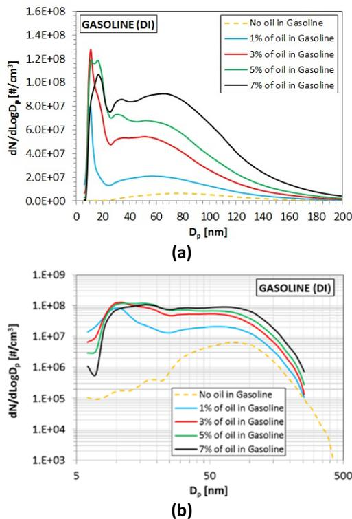
15 **Figure 10** PSD functions (mean values) with mass lubricant oil content equal to 0% (yellow line), 1% (light blue line),
