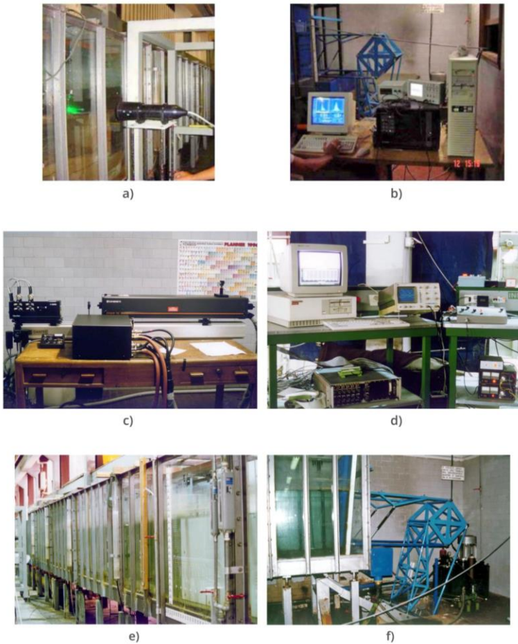
Figure 5: Experimental apparatus: (a) LDA probe; (b) Dantec FVA signal processor and process computer; (c) Laser Coherent Innova and Dantec 2D Fibre Flow optics; (d) process computer with an AD/DA board for the wavemaker control; (e) a part of the wave channel where the jets were discharged; (f) the wavemaker.
