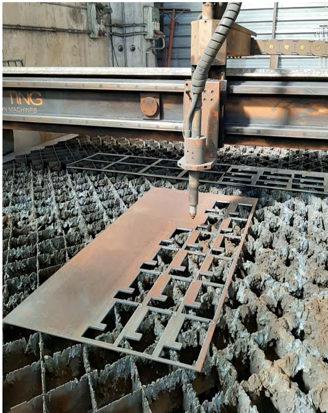
Figure D.1: Precision cut of the connecting hooks to the pantograph
