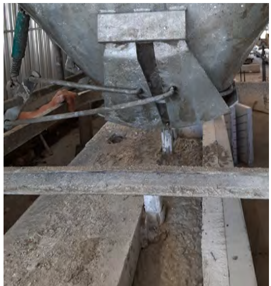
Figure E.47-48-49: LWSC casting through successive layers and with low velocity
