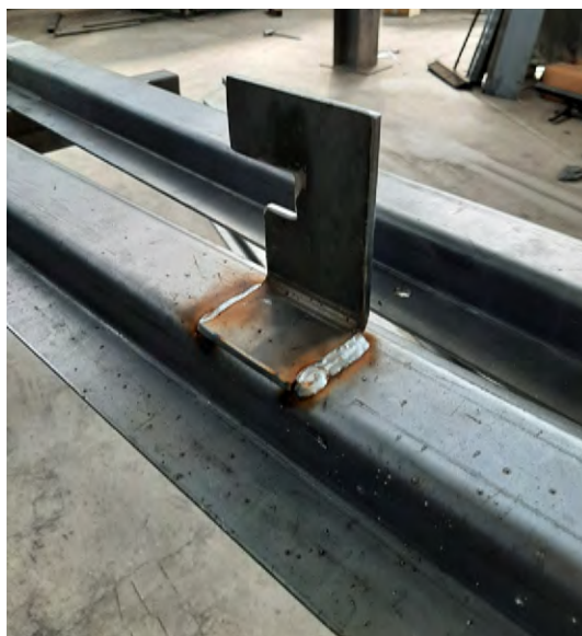
Figure D.9: Hook welding with left folding
