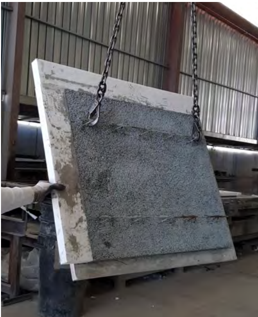
Figure B.29-30-31: Lifting and handling tests of PC modules using a bridge crane
