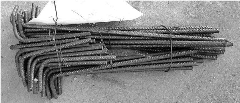
Fig. 6.3-10 – Post-installed rebars. Source: Author
