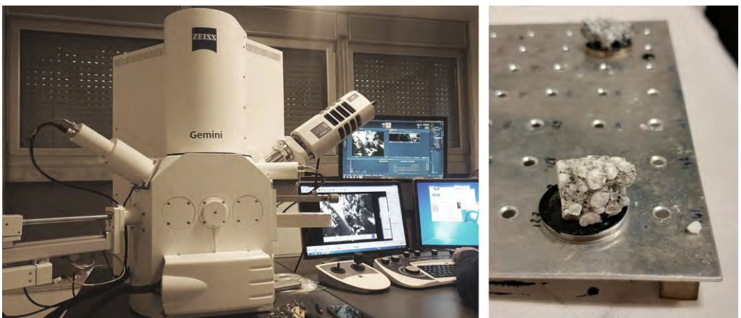
Fig. 4.4-7 - Analysis of mortar morphology and chemical composition by SEM. Source: Author
