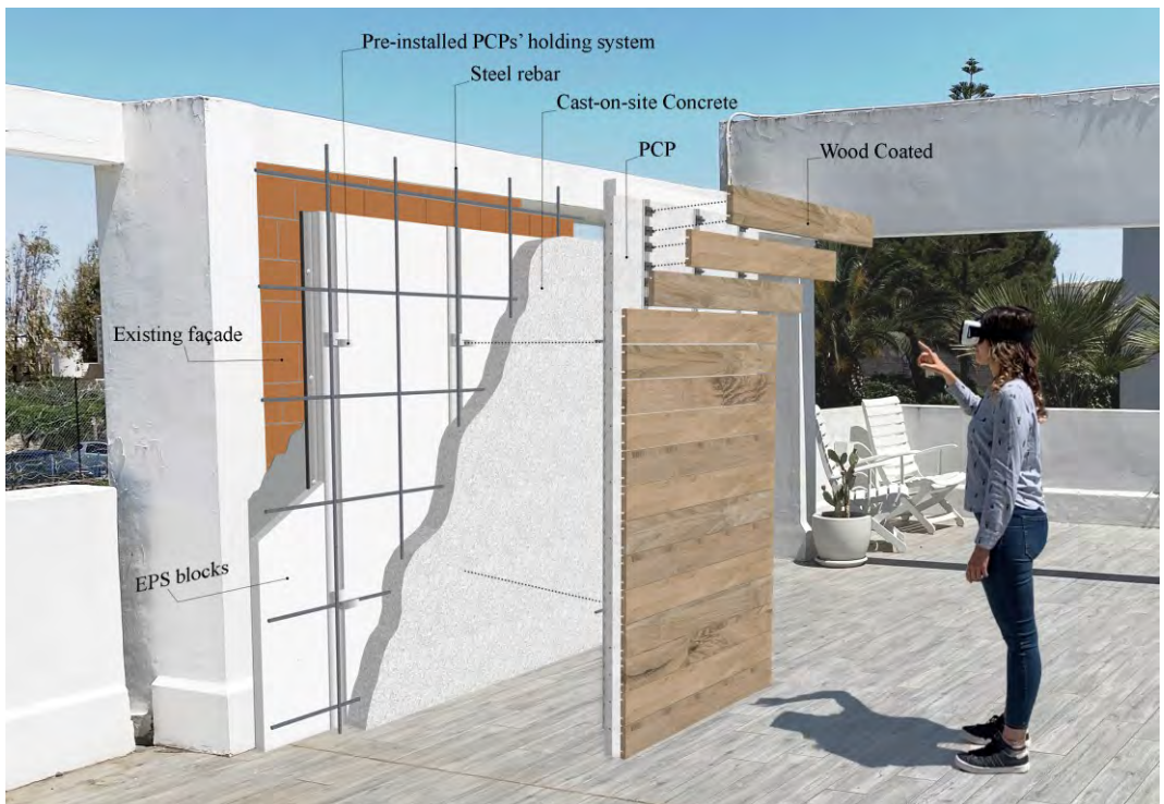
Fig. 5.4-2 – Virtual application on site during the building retrofit displayed in AR. Source: Sangiorgio et al., (2021)
