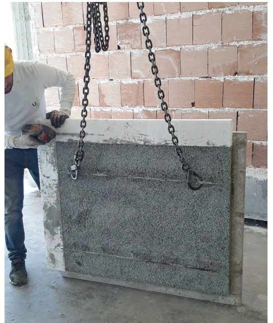
Figure B.29-30-31: Lifting and handling tests of PC modules using a bridge crane
