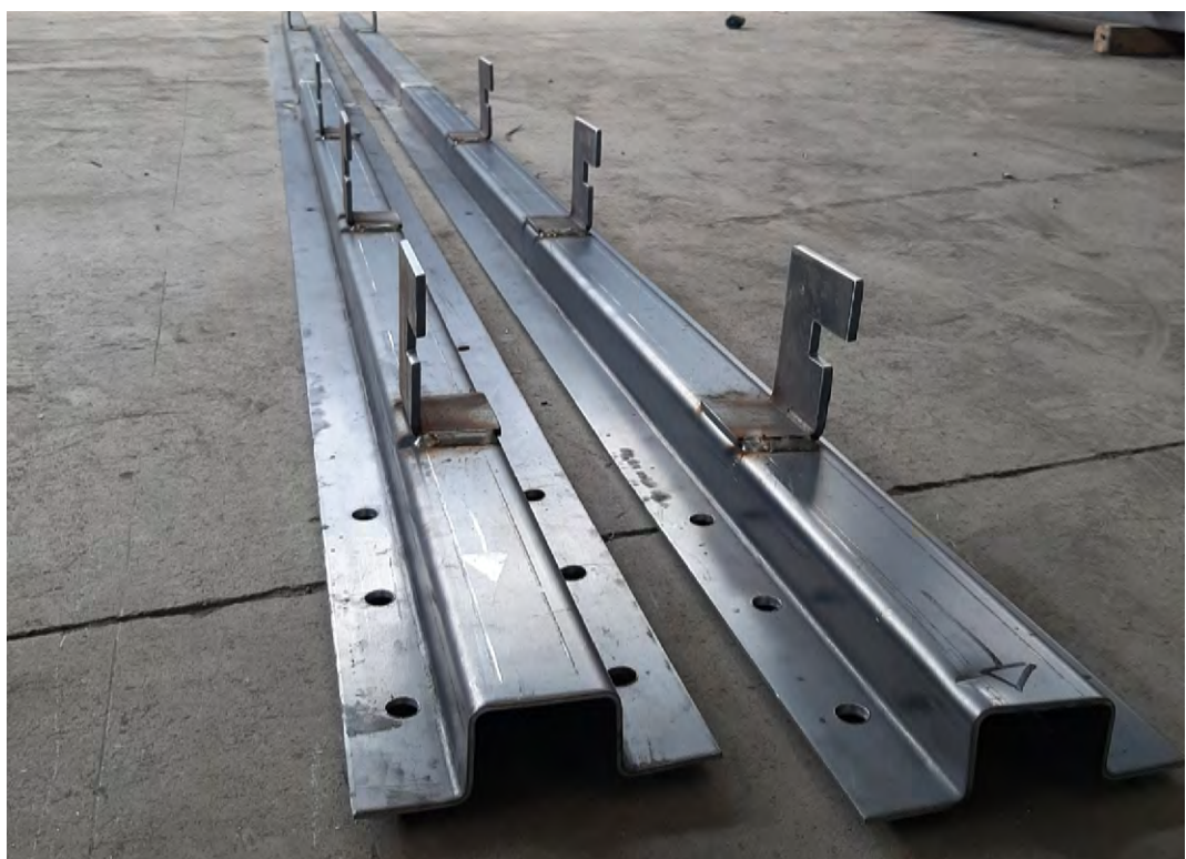
Figure D.11: The couple of mullions for the vertical anchoring of the PC modules
