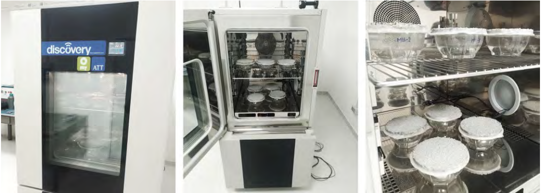
Fig. 4.4-5 - Determination of water vapour transmission properties: wet chamber. Source: Author
