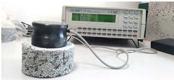
Fig. 4.4-3 - Thermal analysis through the Applied Precision ISOMET 2104 instrument. Source: Author
