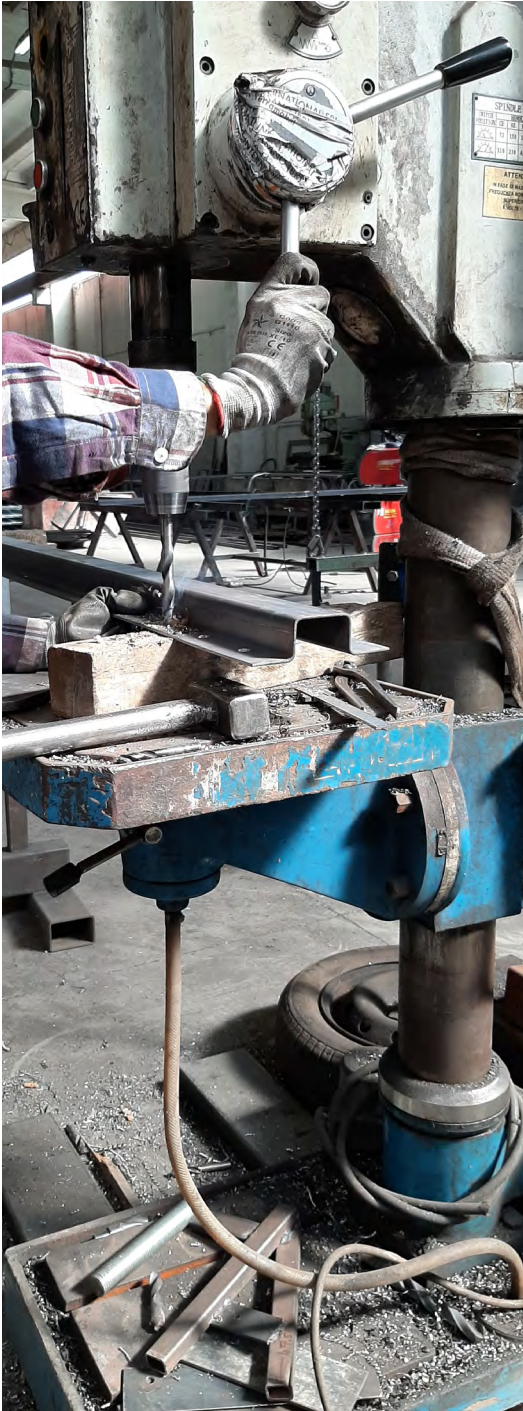
Figure D.6-7-8: Slotting of the mullions according to calculations and design drawings
