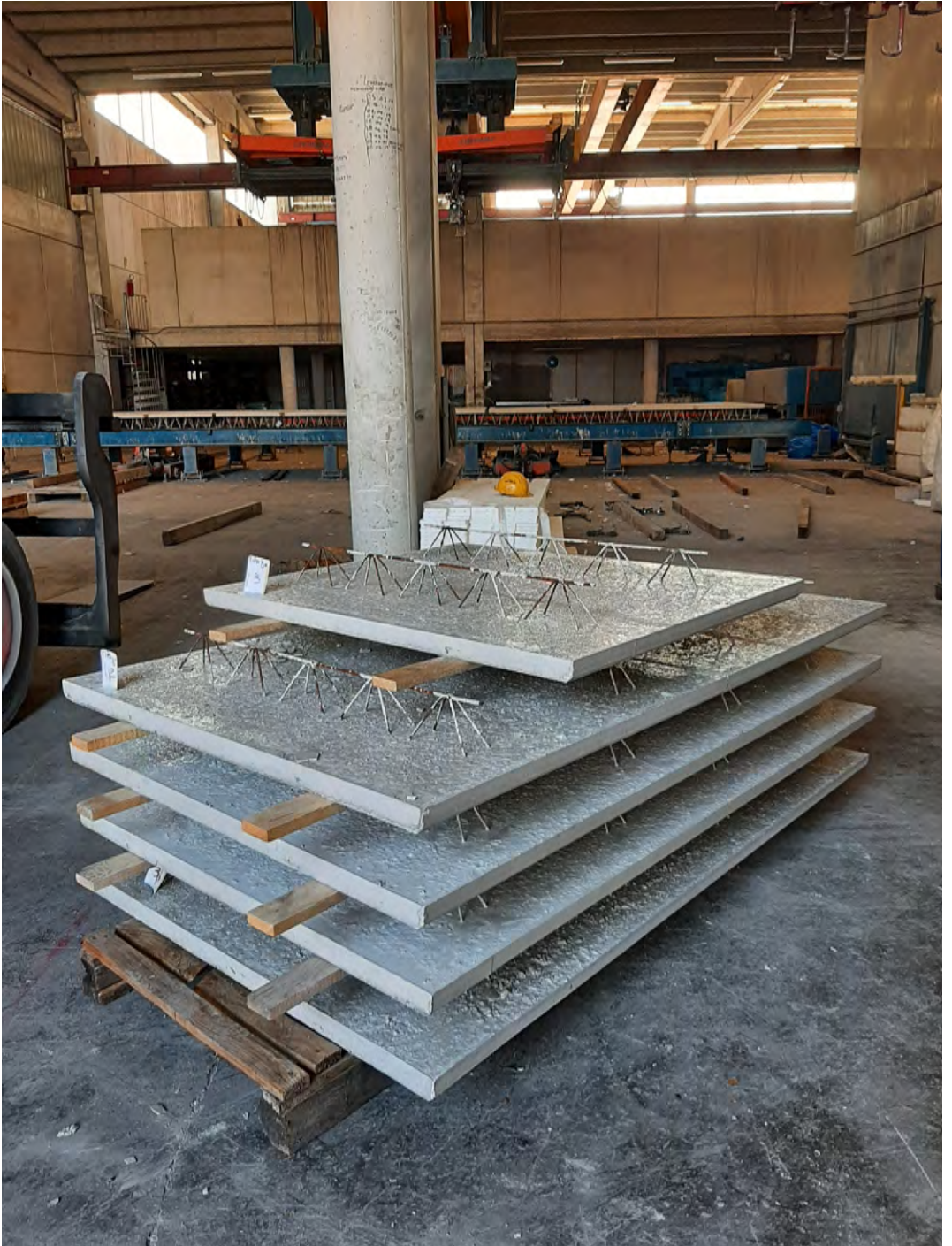
Figure B.14: Form stripping of the base modules
