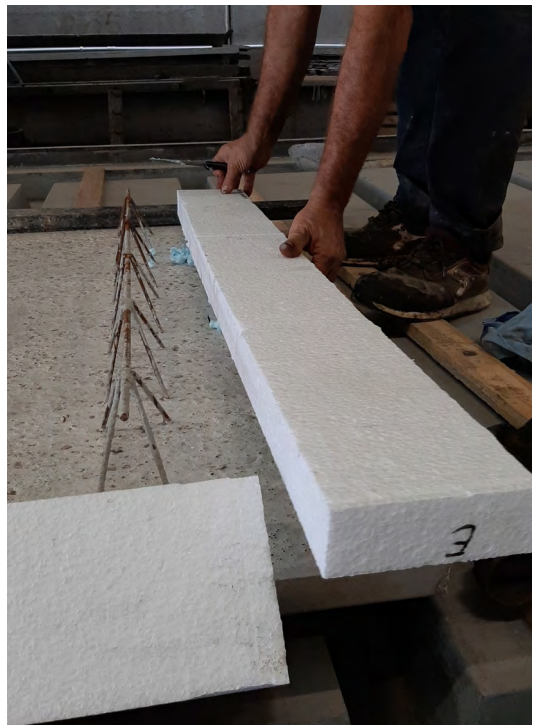
Figure B.15-16-17: Disposition of the REPS blocks on the base modules to generate the male-female joints
