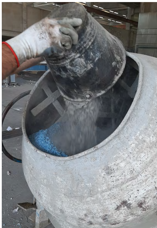
Figure A.5: Cement addition to the additivated rEPS to execute the pre-mixing phase
