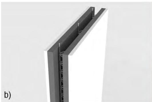
Fig. 3.4-2 - Double layered RC slab: a) for walls; b) HPwalls (with two external layers in EPS); c) for retaining walls. Source: http://www.ferramati.it/web/en/prodotti/double-layered/ (Accessed November 10, 2020)
