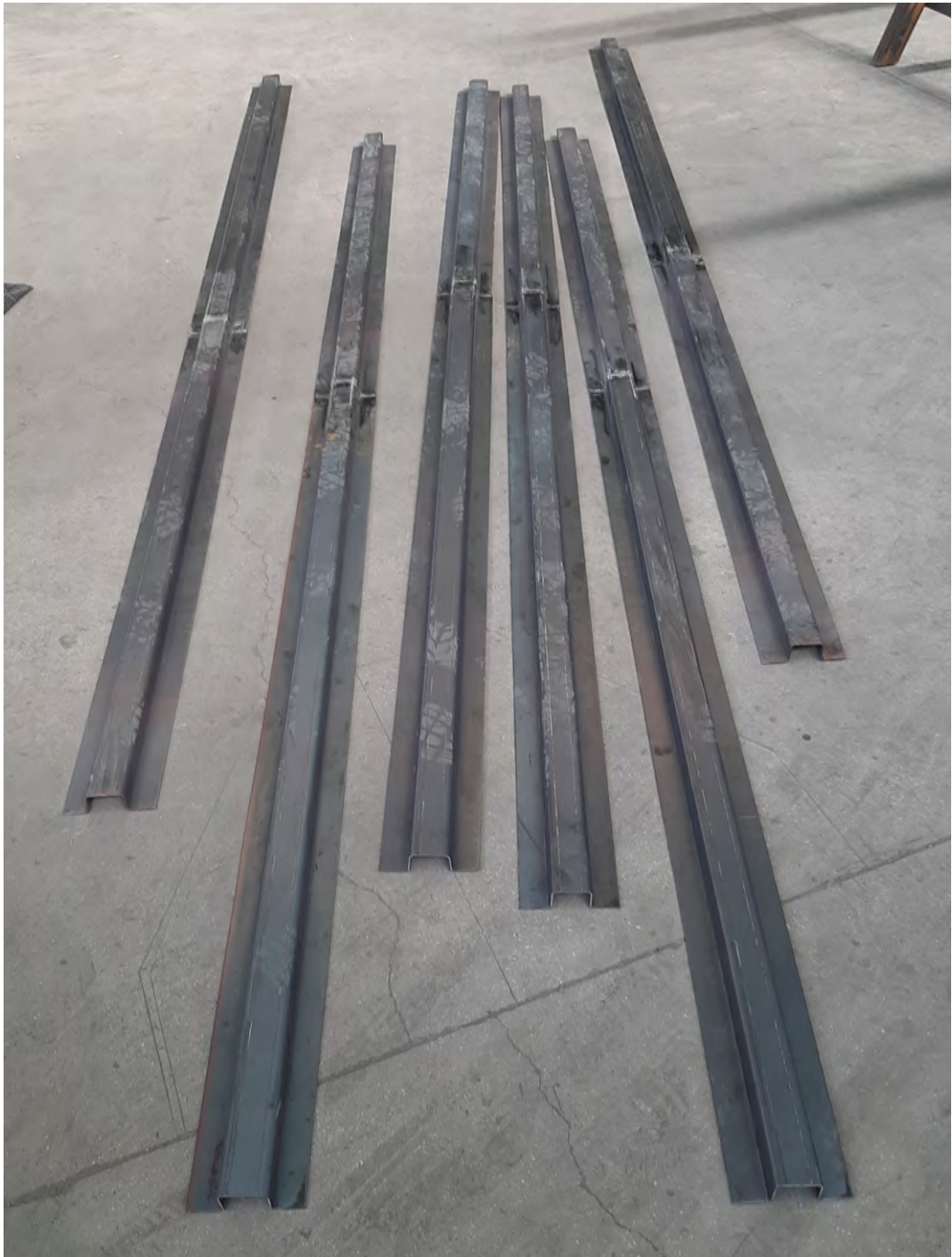
Figure D.5: The three pairs of mullions
