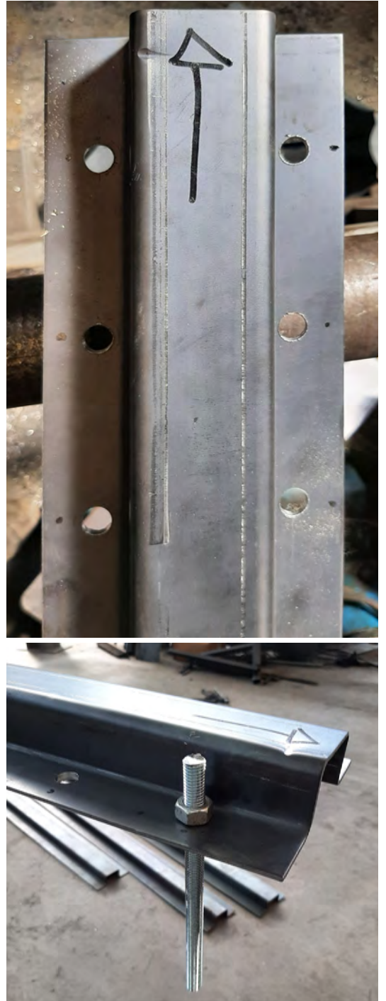
Figure D.6-7-8: Slotting of the mullions according to calculations and design drawings
