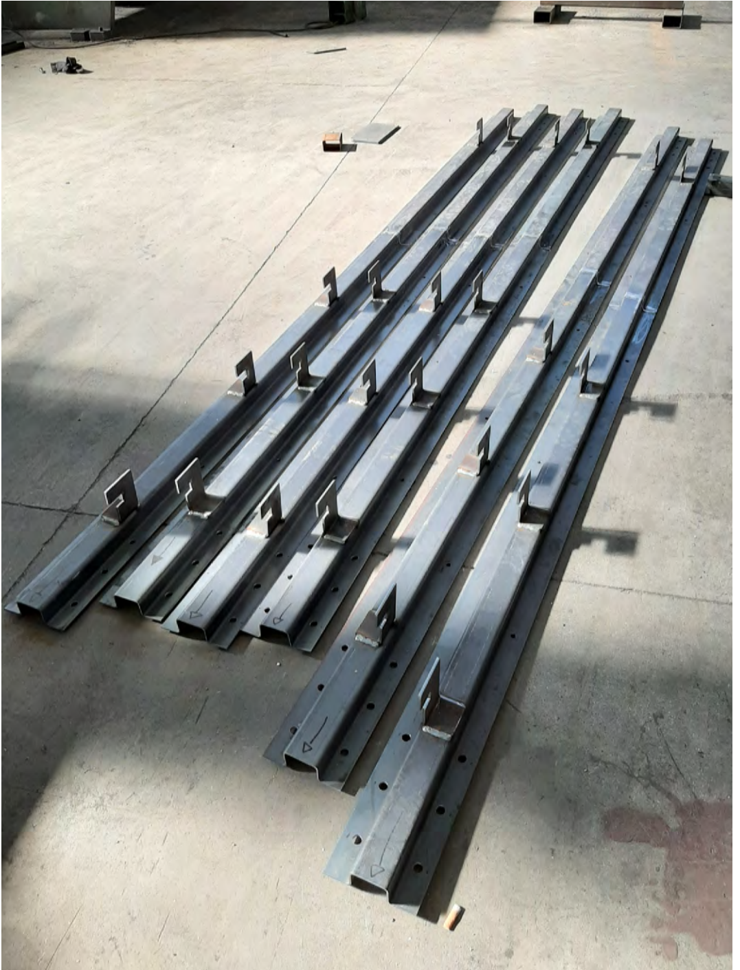
Figure D.12: The three pairs of mullions ready to be anchored on the sample for the system installation
