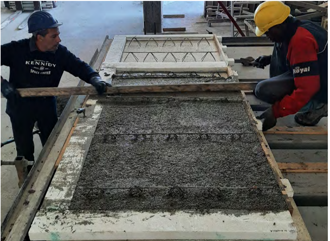
Figure B.23: Surface leveling of the fresh LWM
