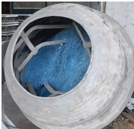
Figure A.1: rEPS additivation in the mixing machine
