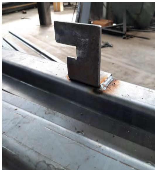
Figure D.10: Hook welding with right folding
