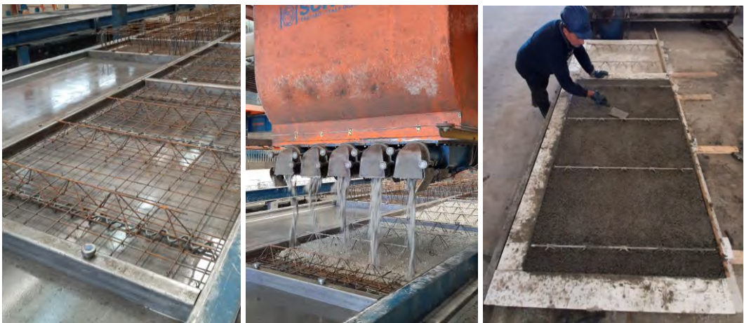
Fig. 6.2-4 – PC module production phases. Source: Author
