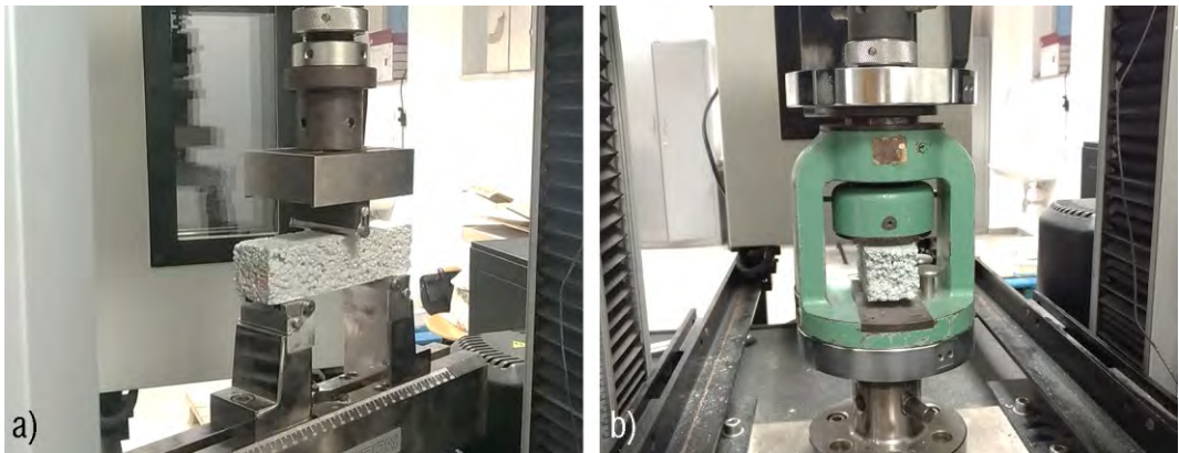
Fig. 4.4-6 - Mechanical resistance tests under a) flexural and b) compressive loads. Source: Author
