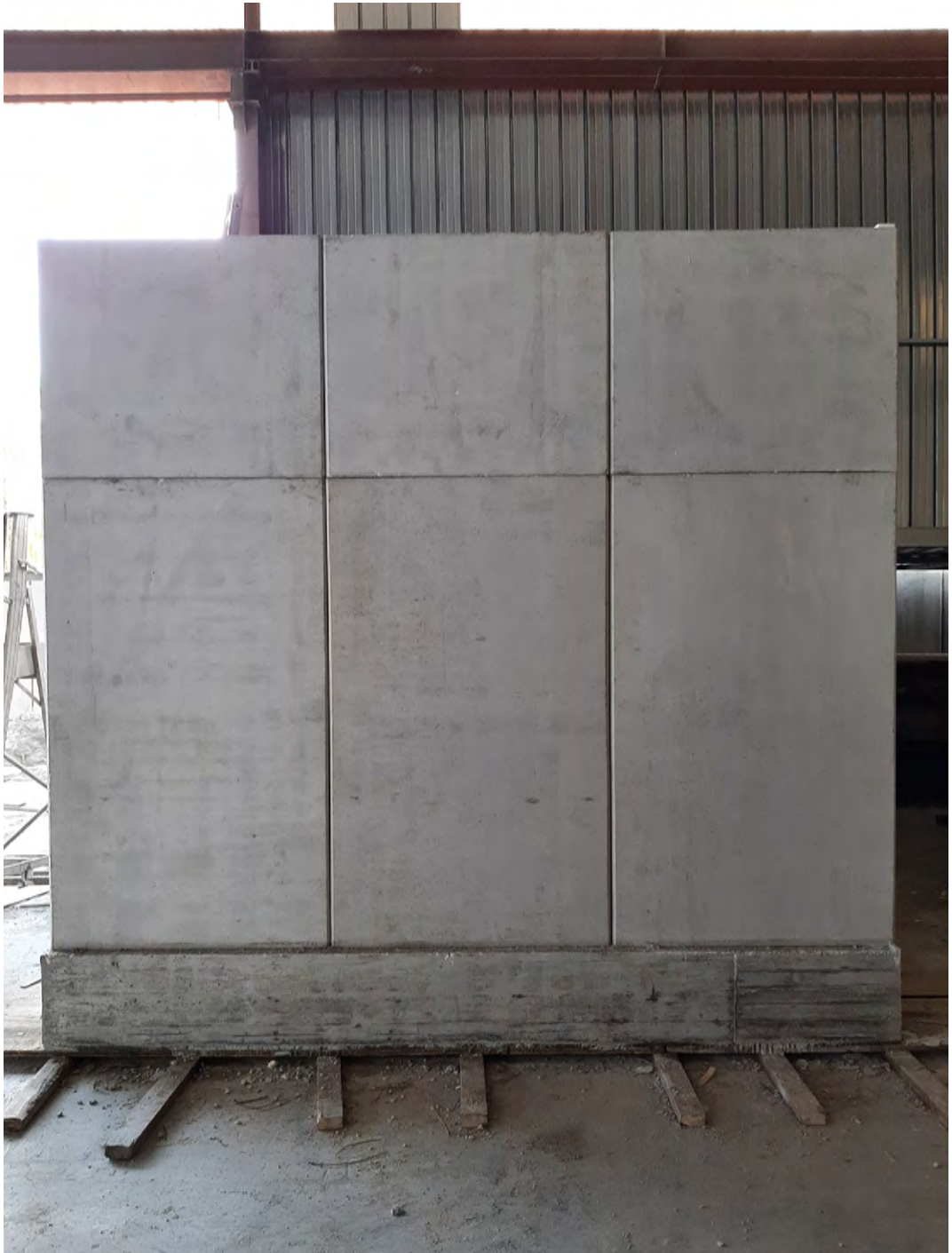
Figure E.53: The model of the “Intelligent PC panel system”: front view
