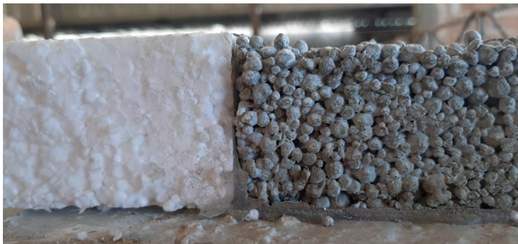
Figure B.27: Junction between the LWM layer and the rEPS block
