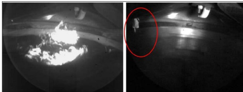
Fig. 2.28 Left: Pool fire on the piston surface due to spray impingement and incomplete evaporation can be a significant source of particle emissions. Right: Soot incandescence from a diffusion flame due to liquid wall film on the injector tip [260].
