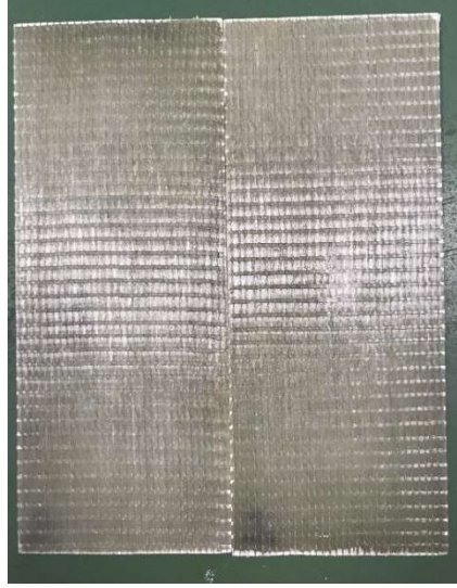
Fig. 7. Damaged GFRP composite samples S1 and S2
