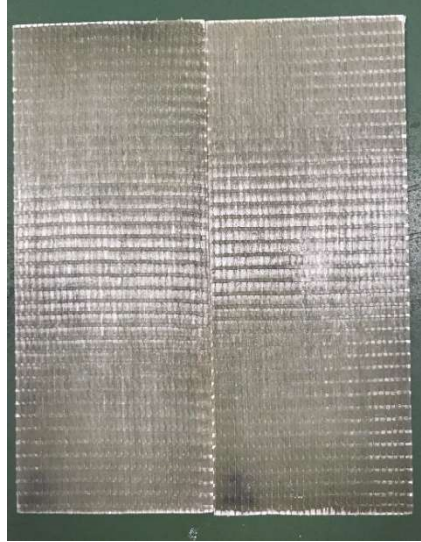
Fig. 7. Damaged GFRP composite samples S1 and S2
