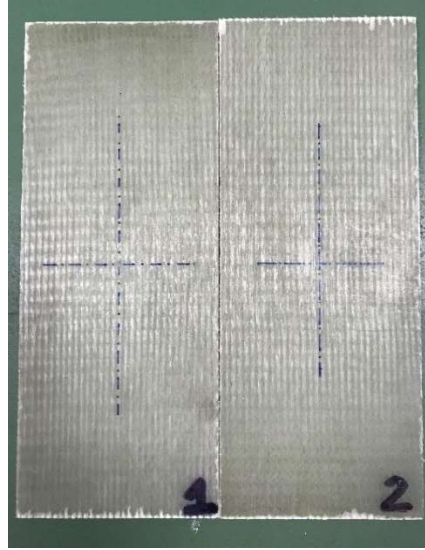
Fig. 5. Undamaged GFRP composite samples S1 and S2
