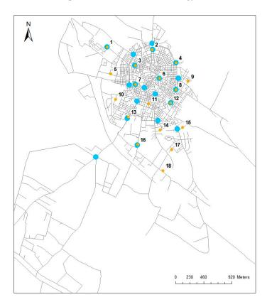
**Figure 5.** Comparison between E-bikes charging stations obtained by the first model (dots in orange) and Pumps used as Turbine (PATs) identified with the second model (dots in light blue).
