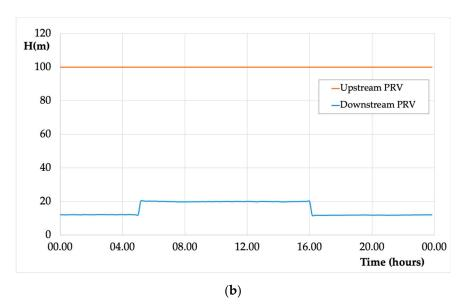
**Figure 2.** Daily flow rate measured for the WDN of the case study (a); Pressure patterns measured upstream and downstream the pressure-reducing valve (PRV) (b).
