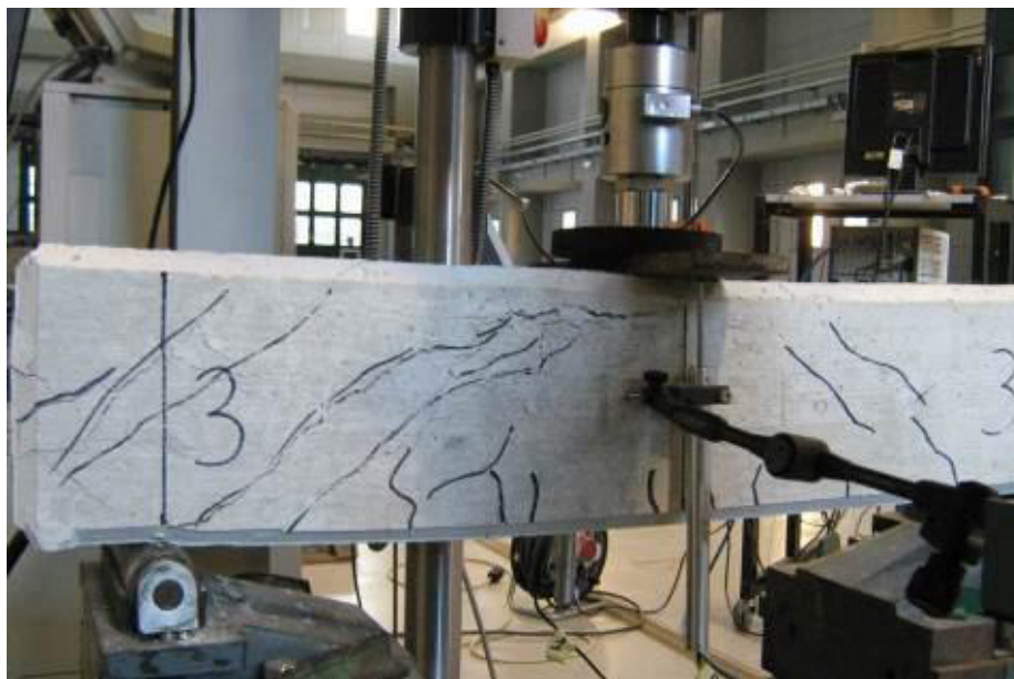
Fig. 14. Cracking patterns on the concrete specimen C20/25 S4 D20 reinforced with CFRP strips.
