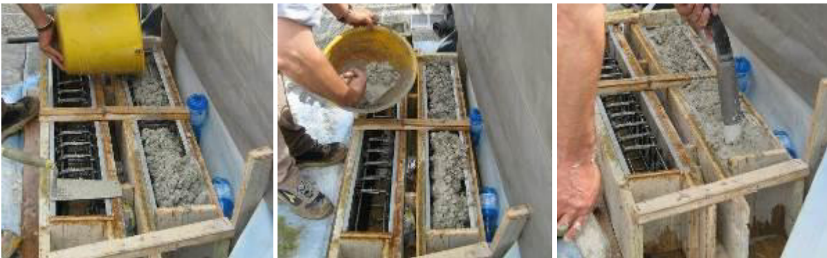
Fig. 5. Phases of realization of the specimens with PET bars.
