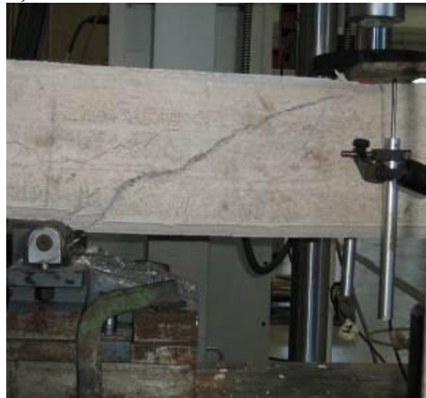
Fig. 10. Detail of the different behaviors; a) specimen reinforced with PET bars; b) specimen reinforced with CFRP strips.
