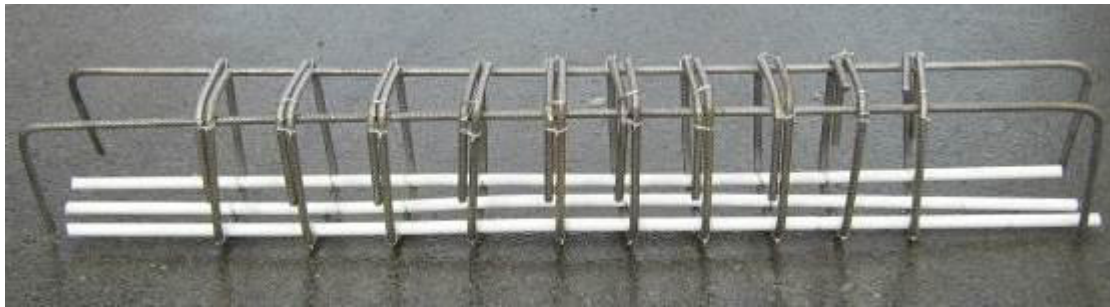
Fig. 4. Positioning of PET bars inside the reinforcing steel cage of the specimen.
