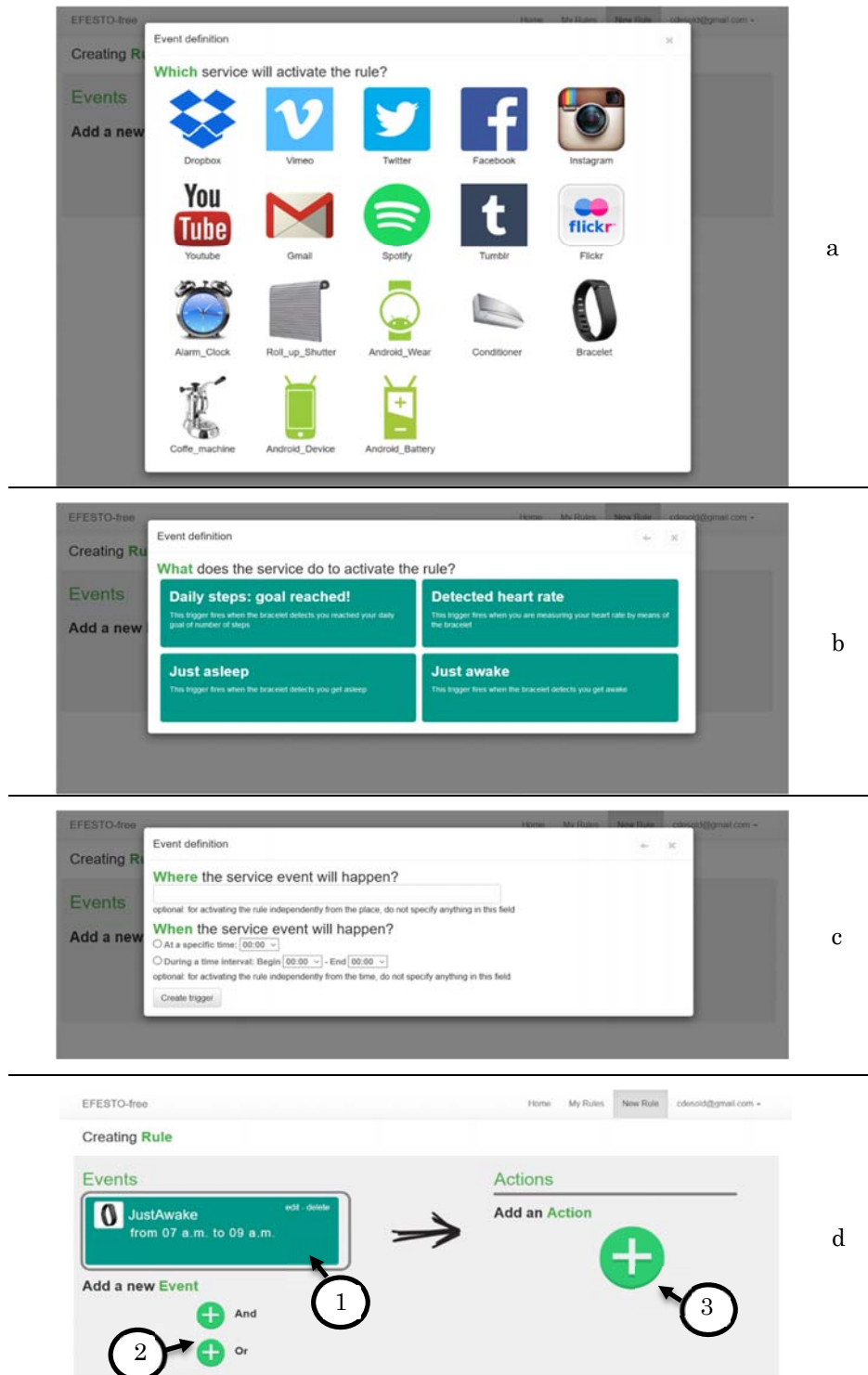
Figure 5. E-Free wizard procedure for specifying events: a) the wizard first asks to select the service that will activate the event; b) as second step, the event is selected among those offered by the chosen service; c) temporal and spatial constraints are defined; d) the event has been defined and the user can define further events or actions.
