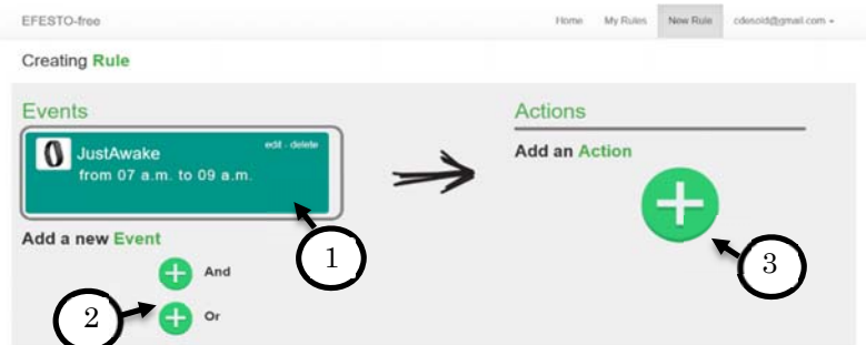
Figure 5.E-Free wizard procedure for specifying events: a) the wizard first asks to select the service that will activate the event; b) as second step, the event is selected among those offered by the chosen service; c) temporal and spatial constraints are defined; d) the event has been defined and the user can define further events or actions.
