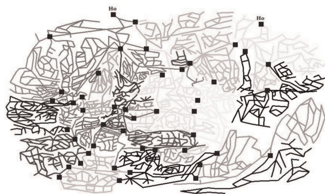
Figure 6. Sampling design configuration corresponding to the maximum value of the sampling-oriented modularity. The black squares represent the locations of pressure meters.
