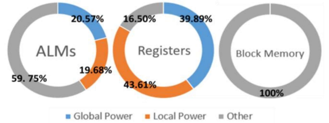
Fig. 9. Contribute in resources utilization of the FSMs that operates in a single EMG branches
