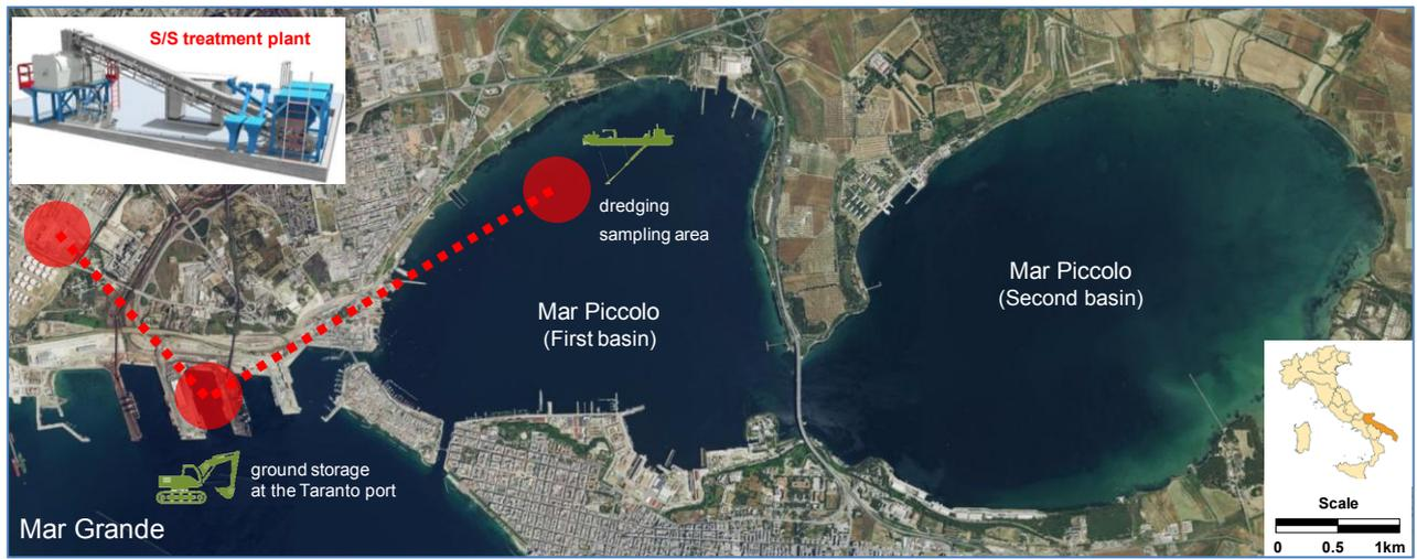
**Figure 1.** The “Mar Piccolo of Taranto” study area (Southern Italy): sampling area, main phases of the intervention (dredging, intermediate storage and treatment) and the S/S pilot treatment plant located at the Taranto Bellavista municipal wastewater treatment plant.
