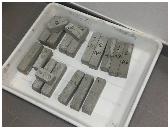
FIGURE 3: DPET-prismatic samples tested to flexural load.
