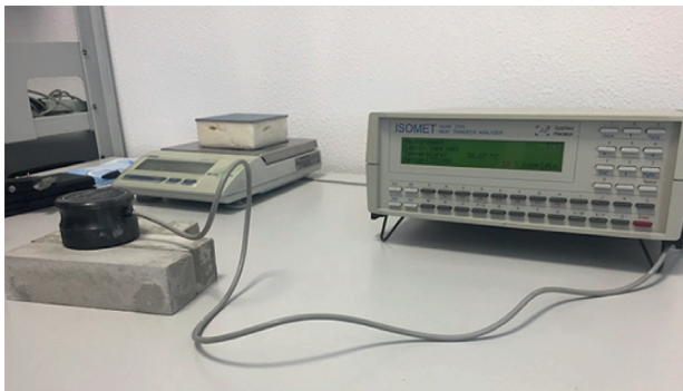
FIGURE 2: Conductivity test device.
