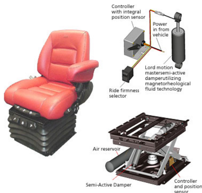
Figure 45. Schematic representation of suspended seats MR dumpers system. [ https://goo.gl/Qas5sZ ; access on 21/11/20].
