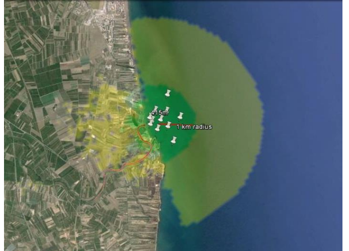
Fig. 14. Coverage simulation around central buoy ("415m" in Fig. 7): green zone has strong signal (Link Margin > 10 dB), yellow zone has weak signal (Link Margin < 10 dB)
