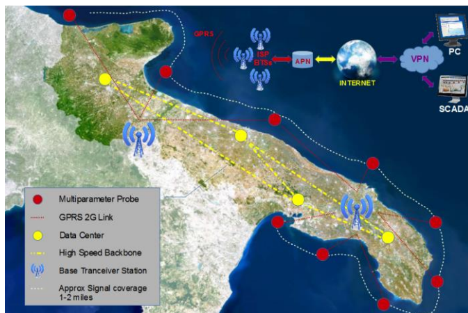
Fig. 15. Conceptual scheme of system architecture superimposed on a satellite image of the Apulia region (ITALY)
