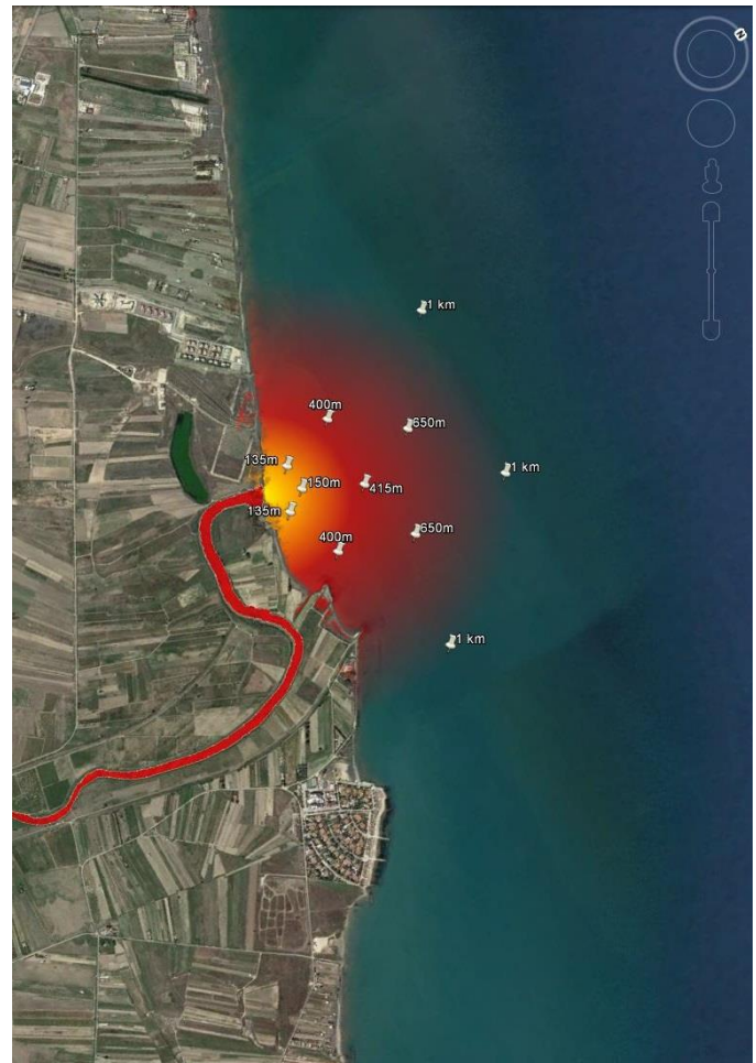
Fig. 7. Transitional water monitoring: Radial probe distribution (white) for impact zone detection. Example of Chlorophyll-a (red) and inverse salinity (yellow) gradient maps that can be obtained.
