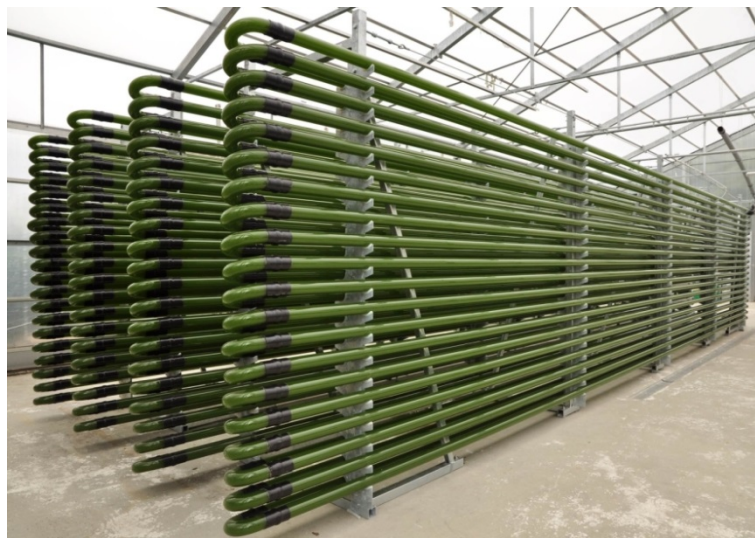
Figure 2: A tubular photobioreactor designated PBR 4000 G IGV Biotech.
