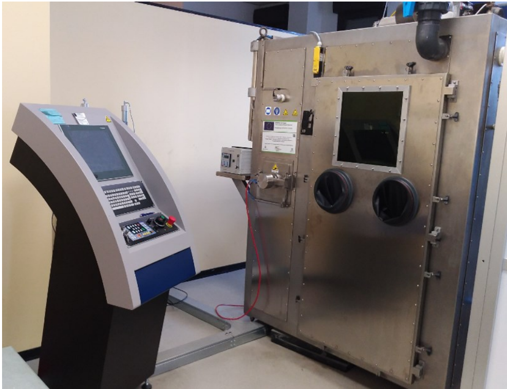
Figure 28 Prototype Direct Laser Metal Deposition system
