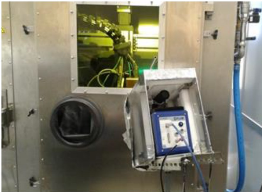
Figure 70 Machine setup and thermal camera device.
