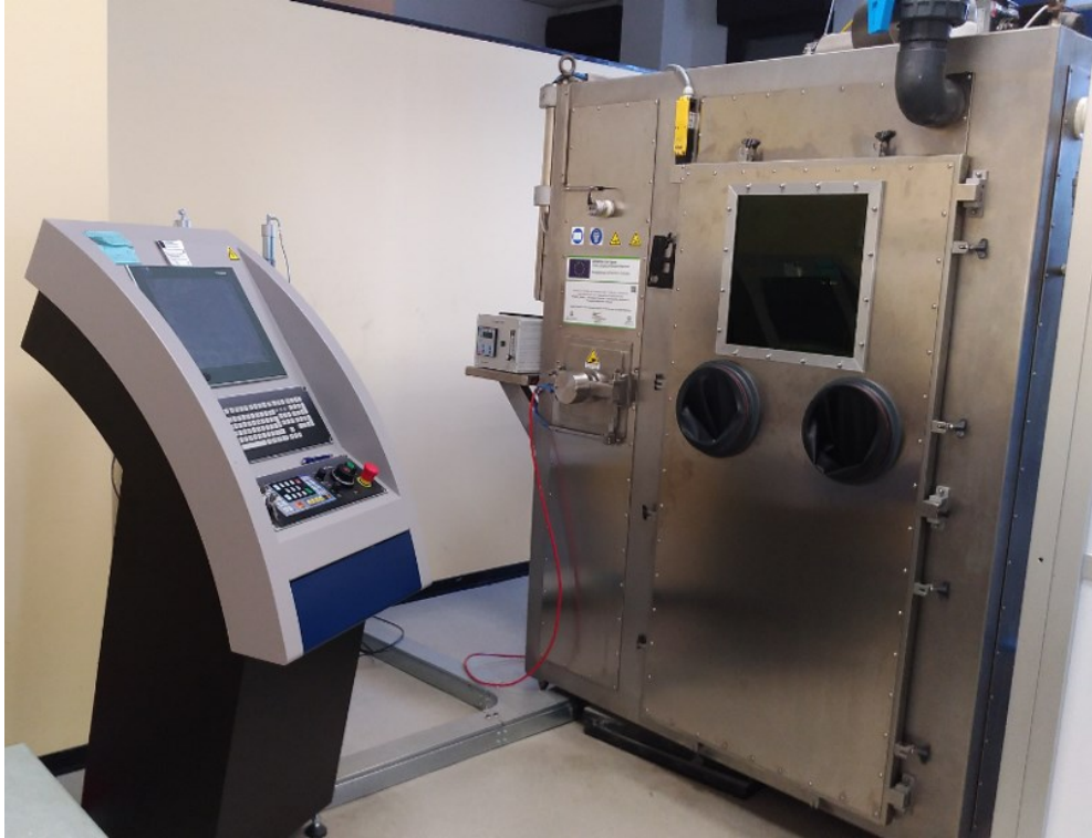
Figure 28 Prototype Direct Laser Metal Deposition system
