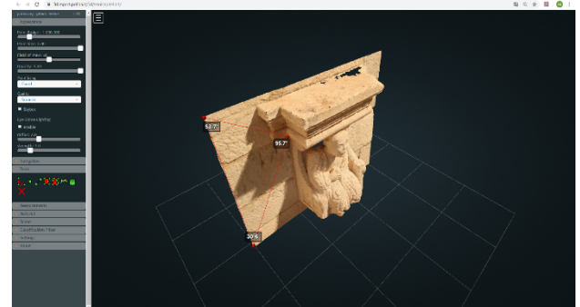
Figure 14. Screenshot, from active “3D” hotspot, showing point clouds of a capital in a web viewer.
