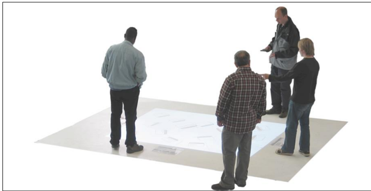
Fig. 8. Using iFloor a group of users can discuss and interact, by using personal mobile phones to write SMSs that are visualized on the floor [Krogh et al. 2004]. Image courtesy of P.G. Krogh.
