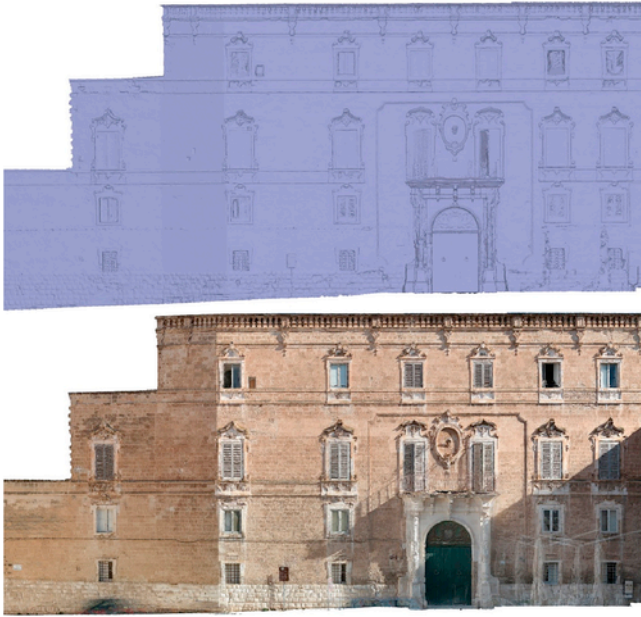
Fig. 2. Three-dimensional models: polygonal meshes with and without texture.
