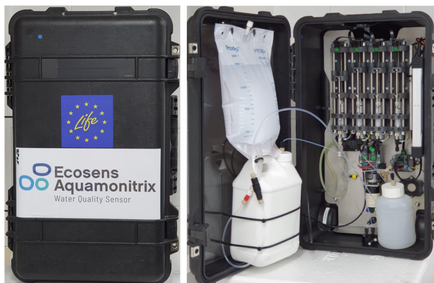
Figure 7. Outer and inner view of an integrated IoT sensor for water quality monitoring applications. The sensor consists of a nitrite and nitrate analyzer based on a novel ion chromatography method, used for detection of toxic substances [112].
