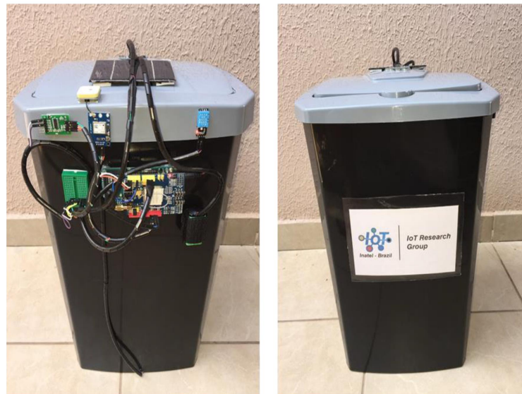
Figure 8. Front and back view of the My Waste Bin, an IoT smart waste container, enabling real-time GPS tracking and weight monitoring [43].
