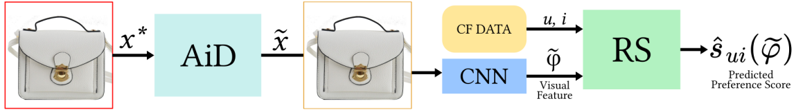
Fig. 6.1 Overview of a Visual-based Recommender Systems protected by the Adversarial Image Denoiser (AiD) in the presence of an Adversarial Image ( x^* ).
