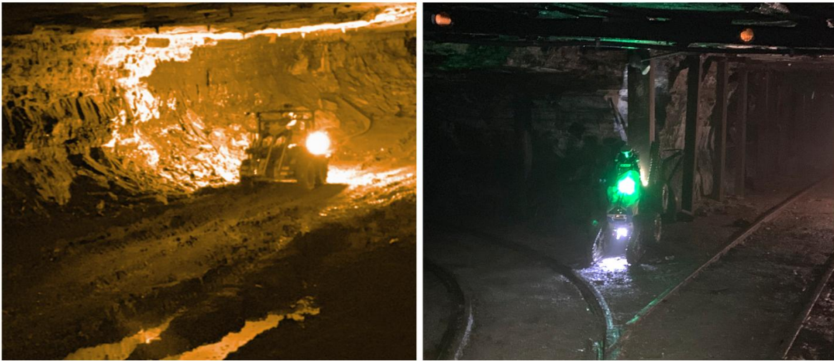
Figure 1.3: Example of hazardous traversability in extreme terrains. On the left, a wheeled platform involved in autonomous subterranean exploration. On the right, a tracked vehicle stuck on a obstacle within hazardous traversal of train rails.
