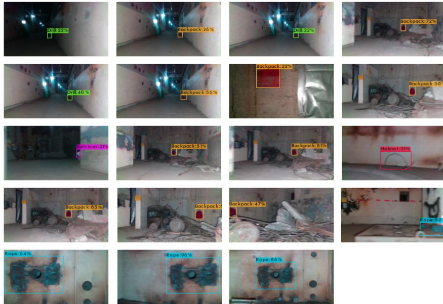
Figure 6.21: YOLO detections on spot1 camera stream when running on-board of the robot with a 50 % downsampling factor.
