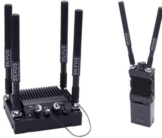
Figure 6.2: Silvus radios used in the mission. Mobile agents can carry multiple communication nodes that are autonomously dropped when a mission-level criteria is met (e.g. low bandwidth and/or signal-to-noise ratio with respect to the base station)
