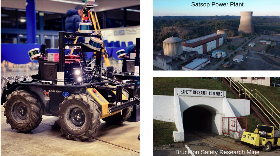
Figure 4.5: On the left, the husky robot used for the autonomous exploration and data collection. On the right, pictures of the circuits where the robot has been deployed within the context of the Tunnel and Urban circuit of the DARPA Subterranean Challenge.
