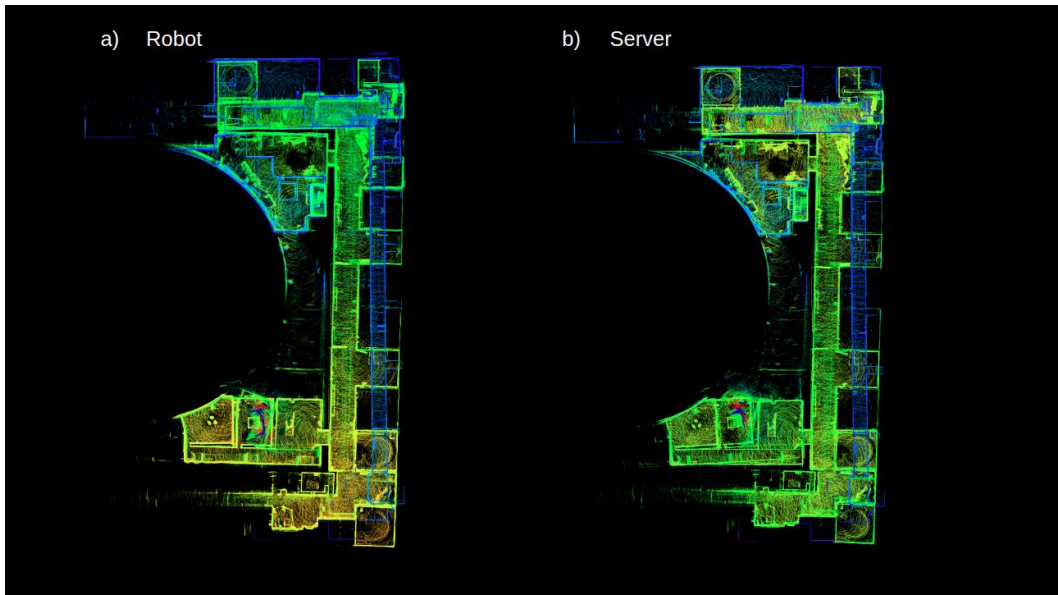
Figure 6.5: Top-view of the maps produced by LOCUS on client (spot1) and server (husky1) for the exploration of spot1 in Urban Beta 2. The server-side computed LOCUS on client's data results in substantially greater accuracy.
