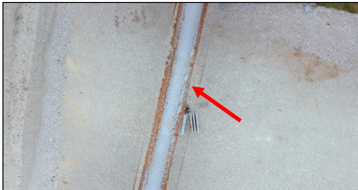
Figure 2.14. Distortions related to the blending mode in PIX4D Mapper software.
