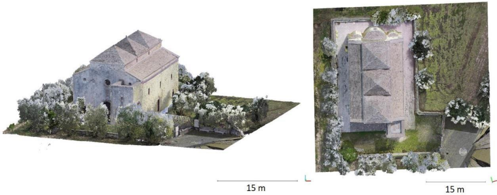
Figure 6.19. Fused model results. XZ and XY perspectives are reported on the left and the right, respectively.
