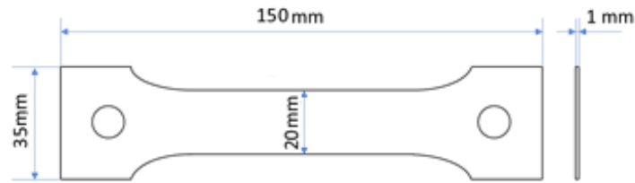
Figure 29 geometry of the specimens used in TSA tests.
