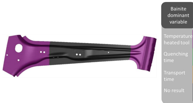
Fig.4.9: Dominant variable that influences bainitic microstructure percentage on the final stamped component
