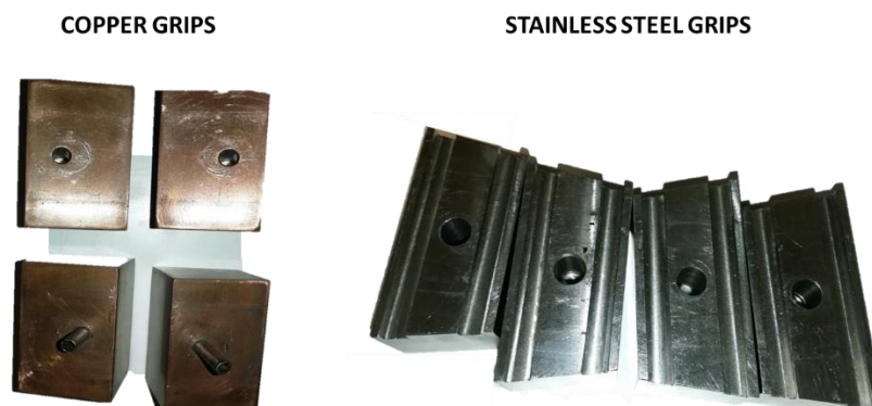
Fig.2.10: Gleeble grips in copper and in stainless steel
