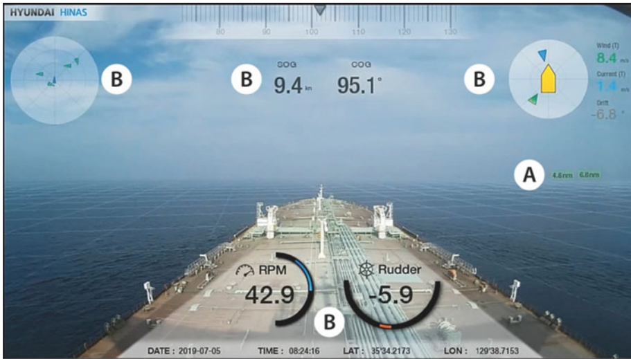
Figure 13. Jeon et al. (2019): AR maritime solution based on HHI Navigation Assistant System (Hi-NAS).
