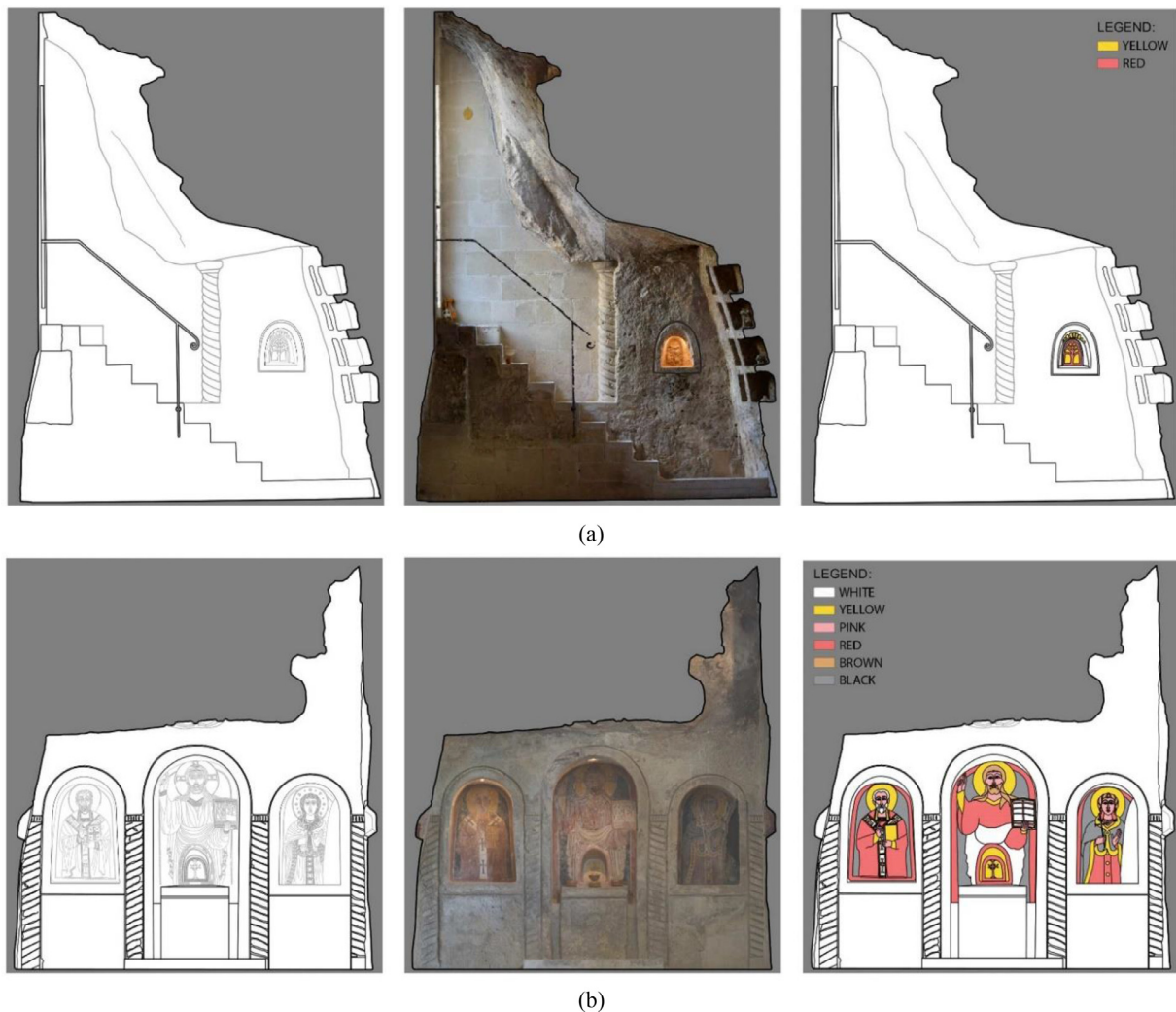
Fig. 4. Orthophotos, CAD representation and colours of the frescoes in the entrance of the rock church (a) and in the wall showing the three religious icons (b).
