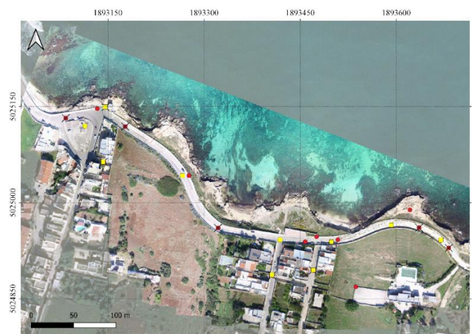
Figure 1. Study area depicted by using the textured orthophoto generated from the photogrammetric datasets acquired on October 16th, 2019, overlapped on a Bing Satellite Map (EPSG:3857 - WGS84/Pseudo-Mercator). Points measured in the GNSS survey campaign in the three analysed scenarios: i) Indirect Georeferencing with 20 GCPs (red dots), ii) Indirect Georeferencing with 10 GCPs (marked red dots), Direct Georeferencing. CPs (yellow dots) in the three scenarios.
