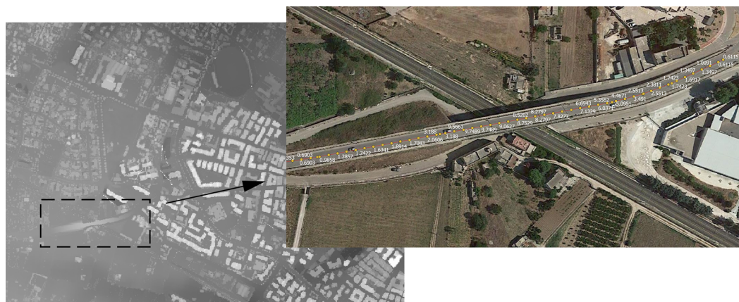
Figure 2.2: Digital Surface Model for the city of Bisceglie (Italy) obtained by using LiDAR data.
