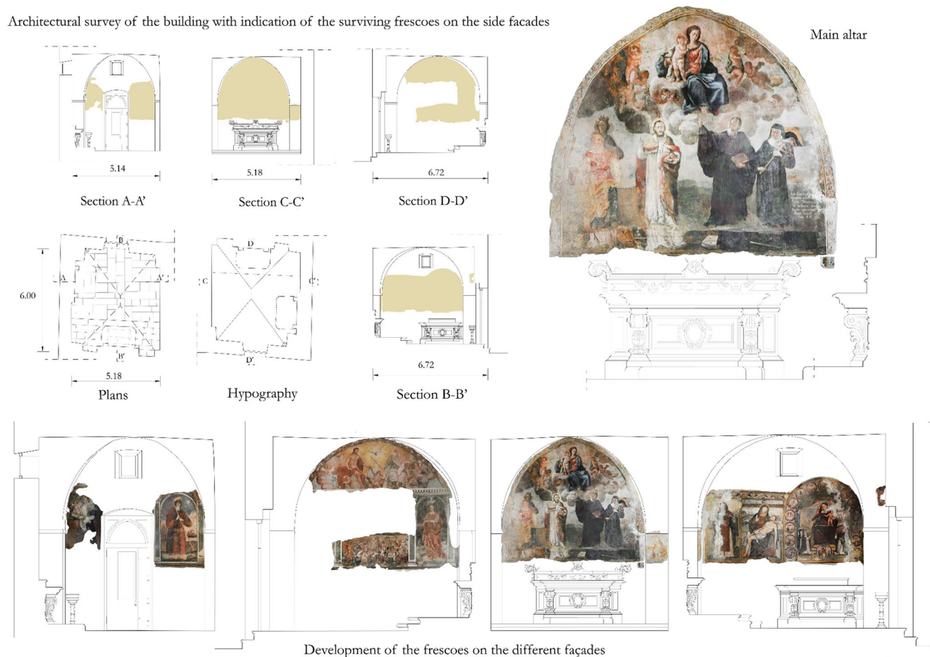
Fig. 6 Architectural layout of the interior of San Nicola in Montedoro church: 2D representation of the structure and objects of particular historical-architectural value, such as frescoes and altars
