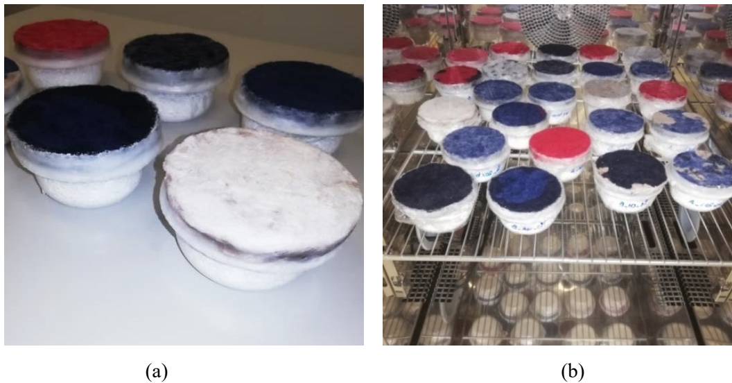
Figure 3.2. Specimens sealed on the top of PVC cups (a) and their conditioning in the climatic chamber (b).
