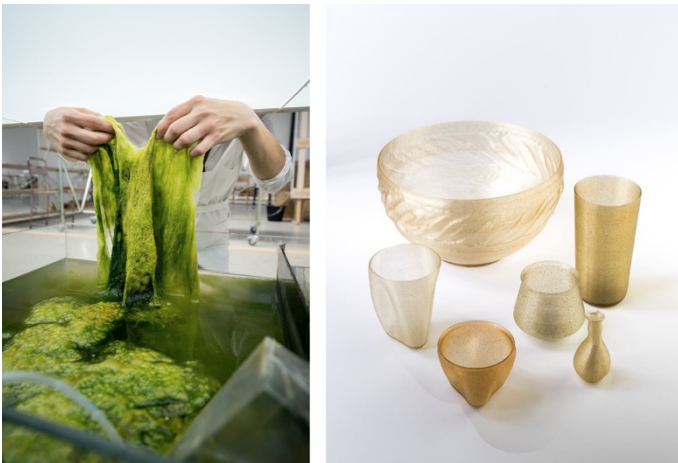
Fig. 2. AlgaeLab (2017) at the Luma Atelier in Arles by Erik Klarenbeek and Maartje Dros. Algae bioplastics and container production through rapid printing. ( www.dezeen.com/2017/12/04/dutch-designers-eric-klarenbeek-maartje-dros-convert-algae-biopolymer-3d-printing-good-design-bad-world )
