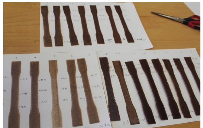
Fig. 6. Samples of 3d-printed Caffil for the stress tests.
