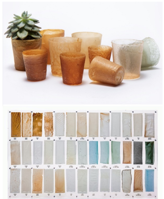
Fig. 1. Shellworks (2019) at the Royal College of Art and Imperial College London by E. Jones, I. Jafferjee, A. Afshar and A. Edwards. Bioplastic based on vinegar and chitin extracted from the shell of crustaceans. Image courtesy: www.dezeen.com/2019/02/22/shellworks-bioplastic-lobster-shell-design
