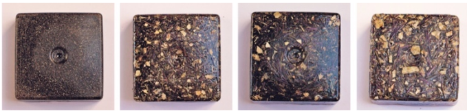
Fig. 13. Echimati: samples with polyester resin based on different grain sizes of the sea urchin shells.
