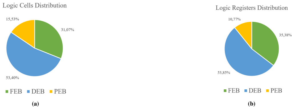
Figure 5.13: PUT post-fitting resources occupancy: (a) combinational function distribution, and (b) register resources distribution.
