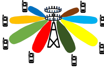
Figure 1.16: Beamforming in mMIMO. Image by Chataut et al. [45]. Image licensed under CC BY 4.0.
