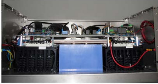
Fig. 11. 30 kW prototype converter used to test the PVs local control.
