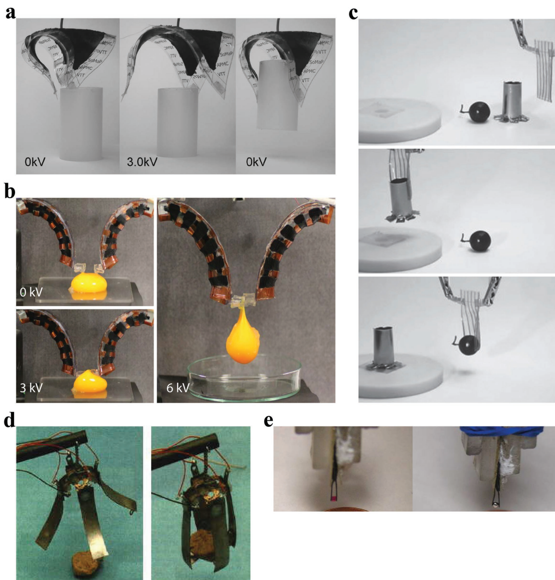
Figure 6. Soft grippers using dielectric elastomer actuators (DEAs) and ionic-polymer–metal composites (IPMCs). a) Dielectric elastomer minimum energy structure (DEMES). Reproduced with permission. [169] Copyright 2007, AIP. b) Segmented DEMES. Reproduced with permission. [171] Copyright 2017, AIP. c) DEA with stiff fibers. [172] d) IPMC fingers. [186] Reproduced with permission. Copyright Yoseph Bar-Cohen. e) Micro-IPMC fingers. Adapted with permission. [187] Copyright 2008, Springer Nature.
