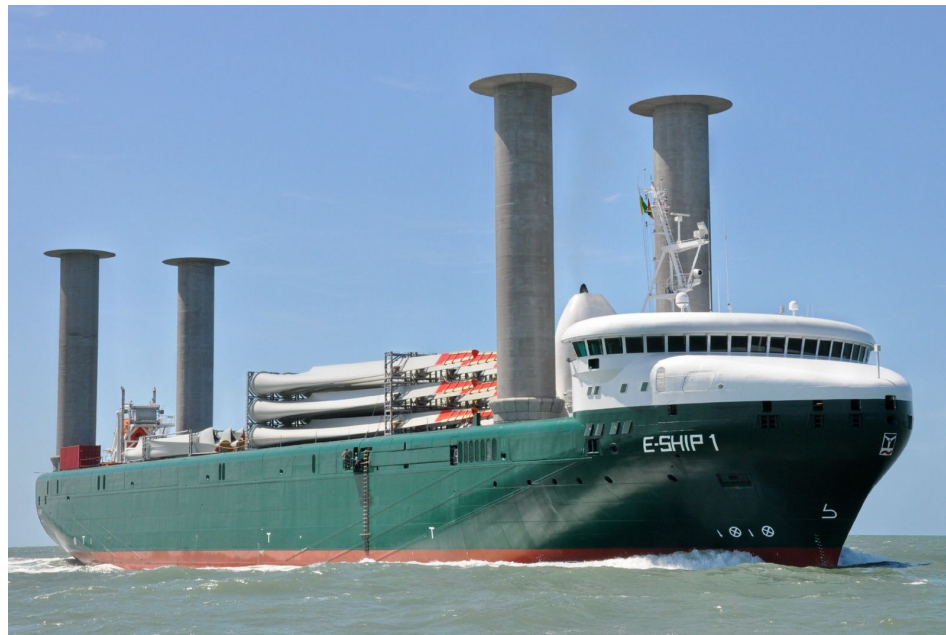
Figure 2.11: E-Ship-1, with 4 Flettner rotors, during the transport of off-shore wind turbine blades
