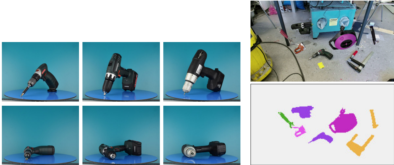
Figure 13: Turntable capture and scene synthesis. Left: Different drills on the turntable as captured by a DSLR camera. Right: Synthetic training scene generated by inserting new objects. The top image shows the resulting color image, the bottom shows generated ground truth for training the segmentation.
