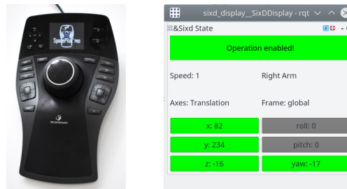
Figure 23: 6D input device (l.) and corresponding GUI (r.) for dexterous wrist control.
