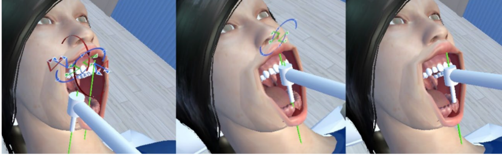
Figure 5.1: Our novel Augmented Collimator Widget (ACW) supports precise 5DOF drill tool positioning in dental implantology. ACW leverages the Gestalt principles, component separation and reification, error visual amplification, and dynamic hiding: approach (left), partial collimation (center), and full collimation, ACW disappears as not needed (right).
