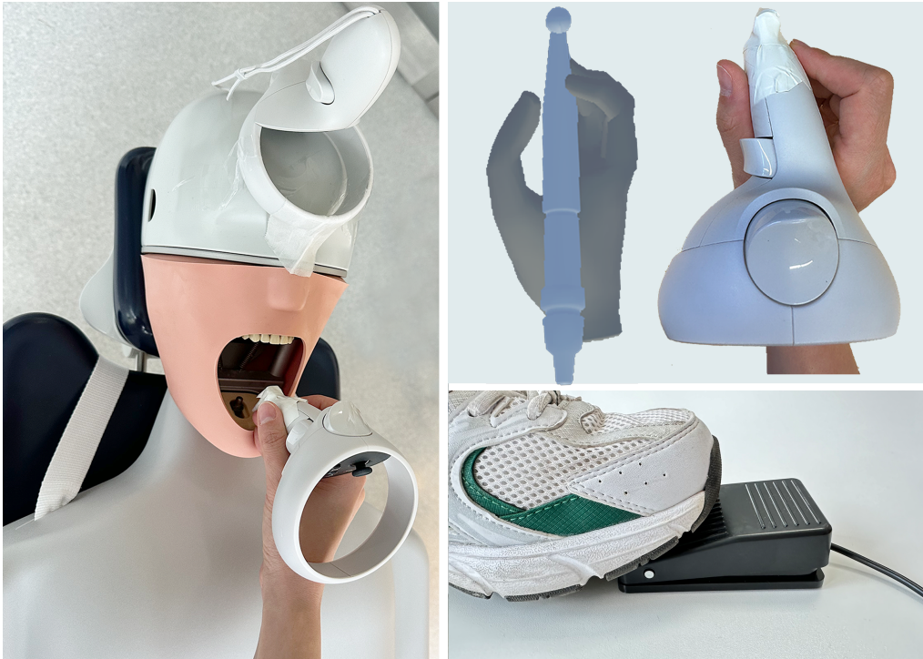
Figure 6.8: Experiment setup; Phantom model tracked with the left controller (left). The right hand is for tool handling (top-right), and the foot pedal is the input device (bottom-right).
