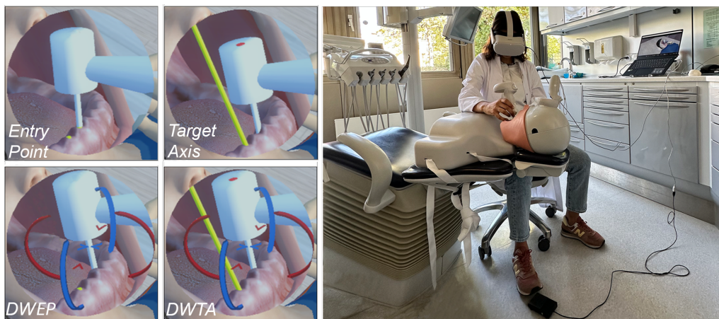
Figure 6.3: Co-designed mixed reality drill positioning widgets: Entry Point, Target Axis, Dynamic widget and entry point (DWEP), Dynamic widget and target axis (DWTA), compared in a realistic setup in the dental room: virtual magnifying loupe (left), tracked phantom and virtual patient, foot pedal, laptop and headset (right).
