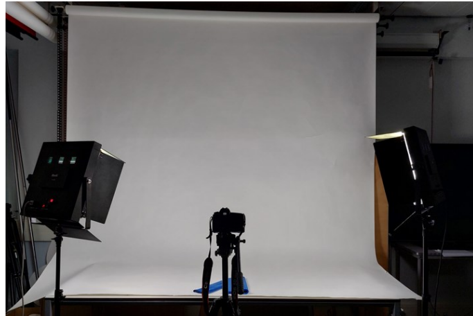
Figure 41. A photographic setup consisting of 2 LS-1200 LED Panels, Canon EOS 5D Mark II on a tripod, a white paper backdrop, and a blue velvet fabric (32 x 46 cm).
